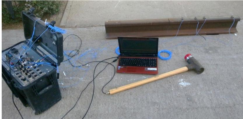
Fig. 1 Experimental modal test setup
