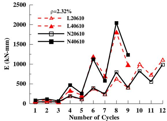
Fig. 15 Energy dissipation versus load cycles ( $\rho=2.32\%$ )
