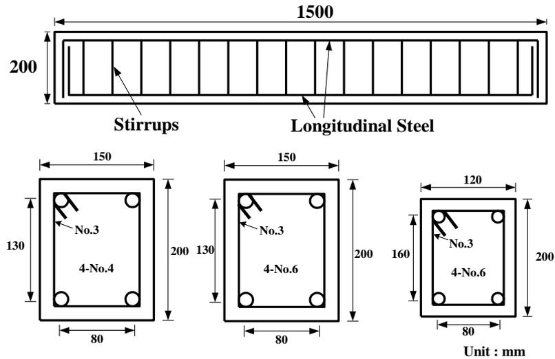
Fig. 1 Specimen details
