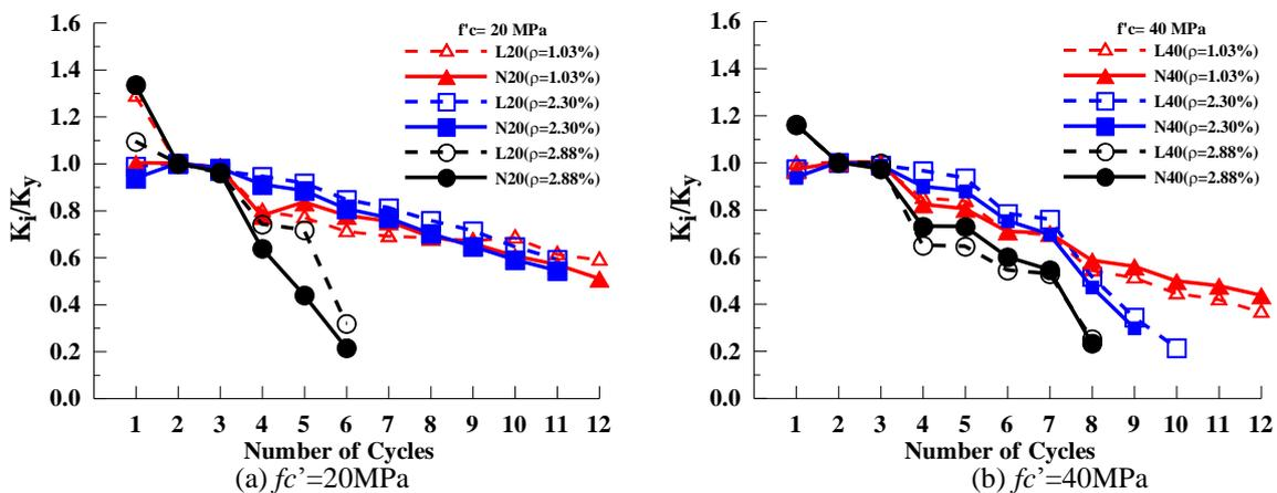
Fig. 12 Effect of tension reinforcement on the stiffness degradation of beam
