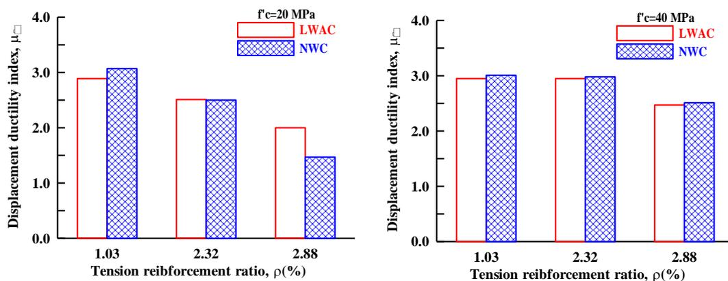
Fig. 7 Displacement ductility index versus tension reinforcement ratio
