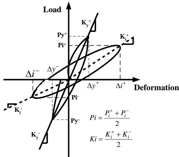
Fig. 8 Definitions of strength and stiffness
