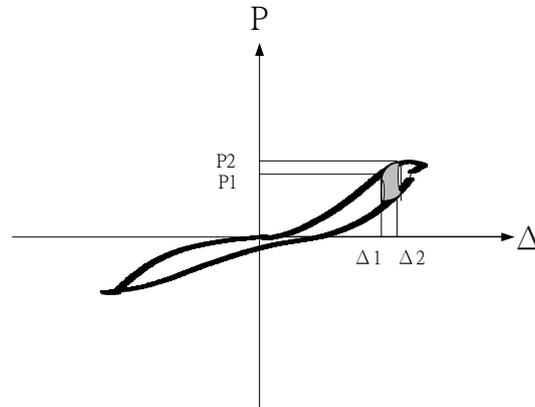
Fig. 13 Calculation of the energy dissipation capacity
