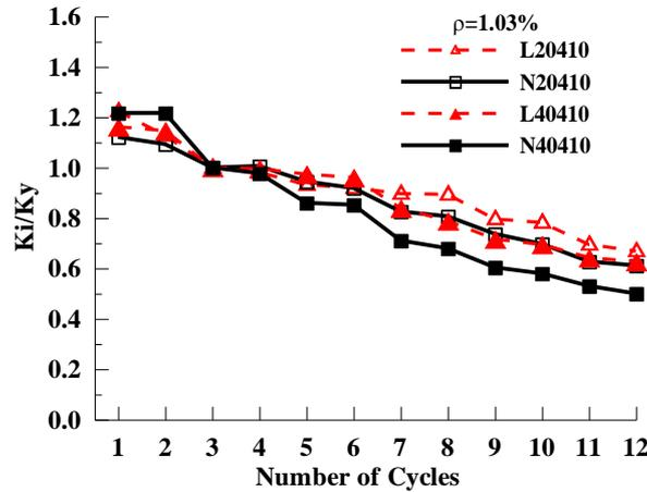
Fig. 10 Effect of concrete strength on the stiffness degradation of beam
