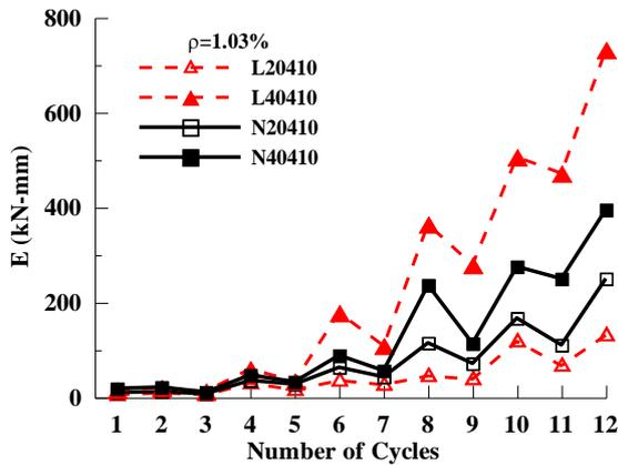
Fig. 14 Energy dissipation versus load cycles ( $\rho=1.03\%$ )
