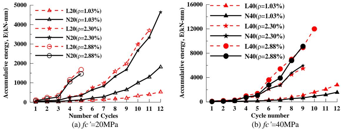
Fig. 16 Effect of tension reinforcement on the energy dissipation of beam
