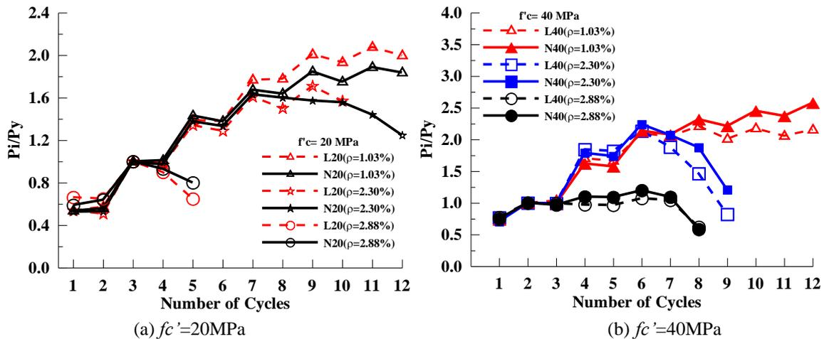
Fig. 11 Effect of tension reinforcement on the degradation of the flexural strength of beam
