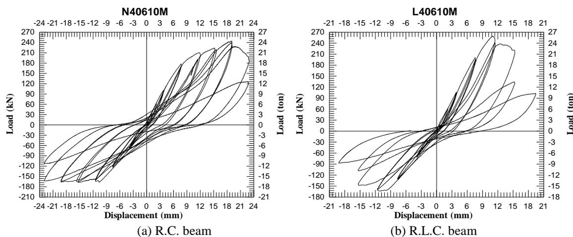
Fig. 5 Cyclic responses of concrete beam
