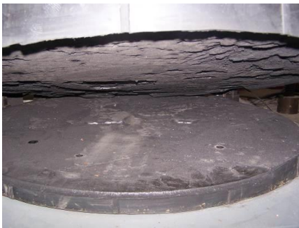
Fig. 14 Crack of the rubber layer for LNR-1
