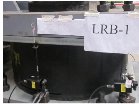
Fig. 15 Crack of the rubber layer for LRB-1
