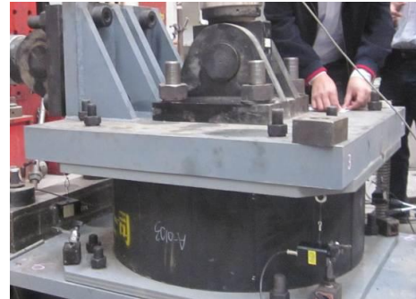
Fig. 13 Rubber bearing test
