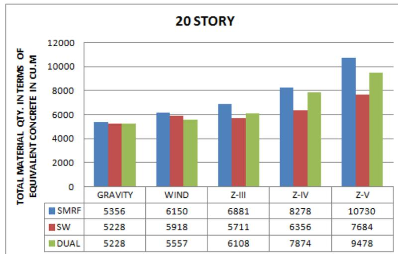
Fig. 7 20-Story total material quantity in terms of equivalent concrete in Cu.m
