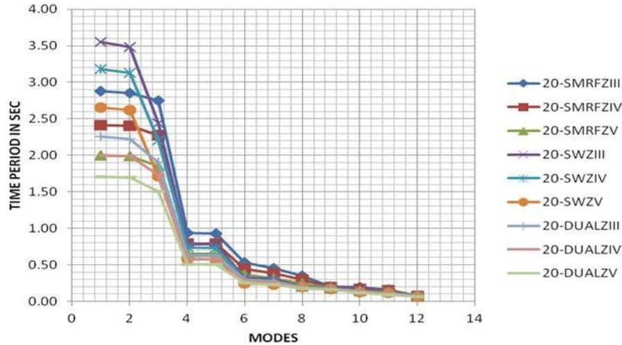
Fig. 4 Time period Vs Modes for 20 Story structures for various lateral load resisting systems
