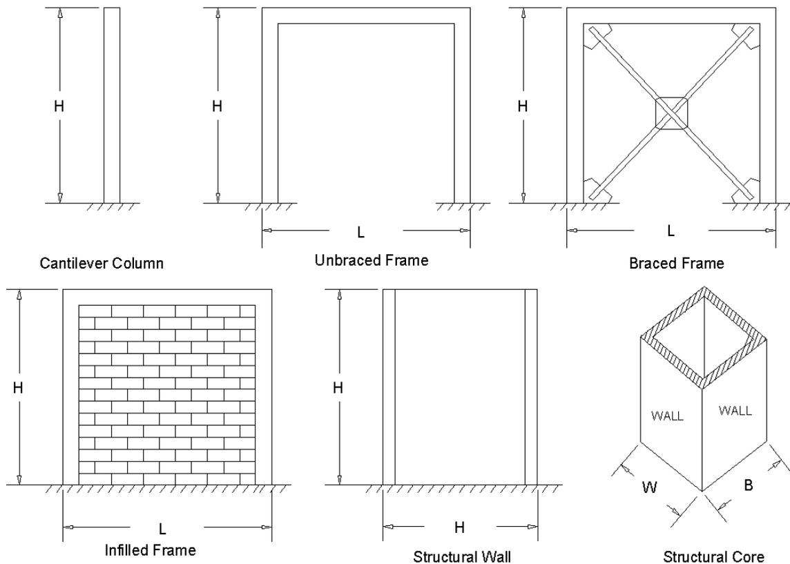
Fig. 1 Basic structural systems with increasing lateral stiffness (from top left to bottom right)
