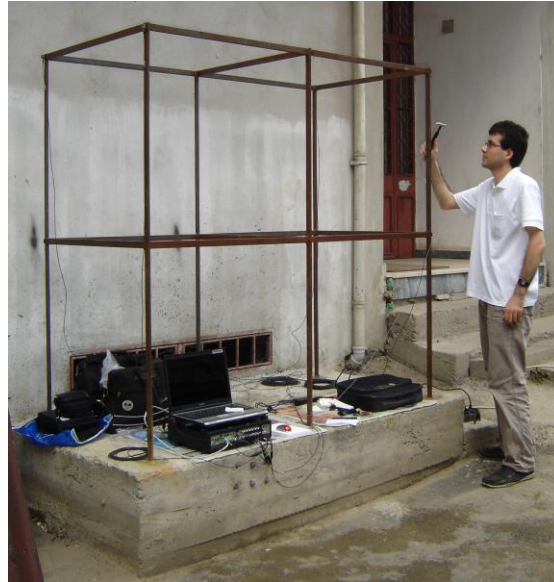
Fig. 10 The 3d frame is excited with a hammer
