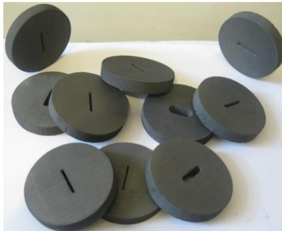
Fig. 2 The UNBD graphite specimens fabricated (not polished)
