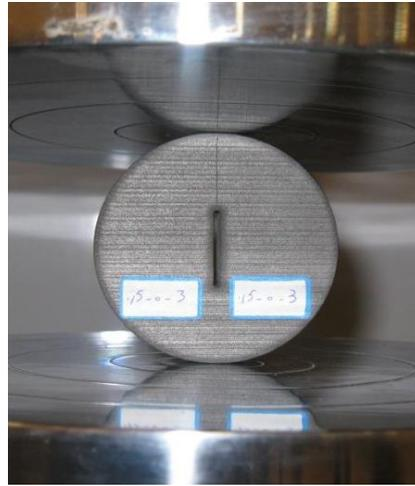
Fig. 3 The UNBD graphite specimen during mode I fracture test
