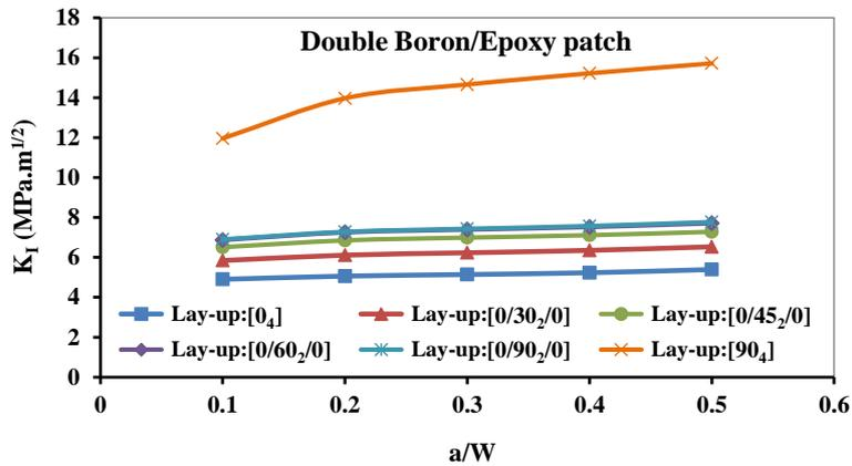
Fig. 10 Effect of double symmetric Boron/Epoxy repair ply orientations on the SIF
