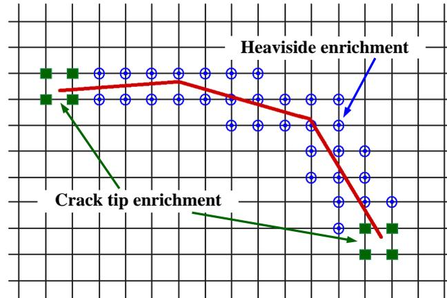
Fig. 1 Enriched nodes in the XFEM: Circles- nodes with 2 additional DOFs, Squares- nodes with 8 additional DOFs (Giner *et al.* 2009)
