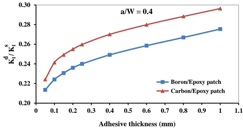
Fig. 7 Effect of adhesive thickness on the SIF (single and double sided repair)
