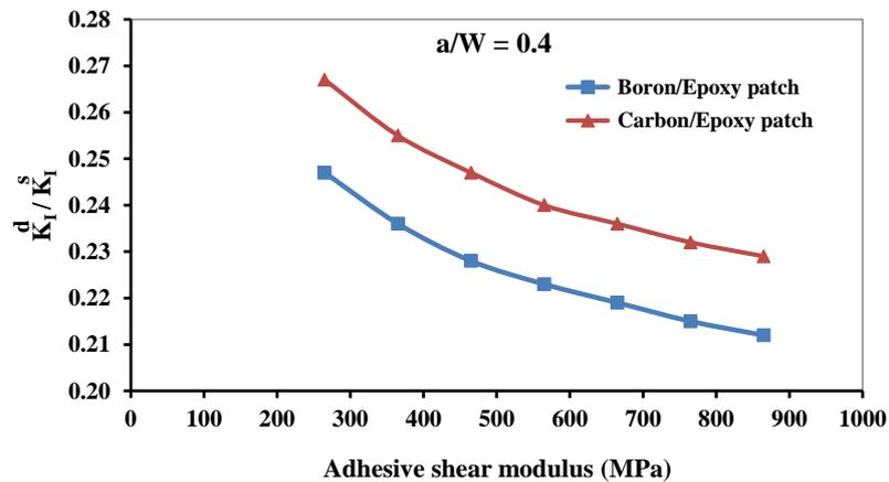
Fig. 8 Effect of adhesive shear modulus on the SIF (single and double sided repair)
