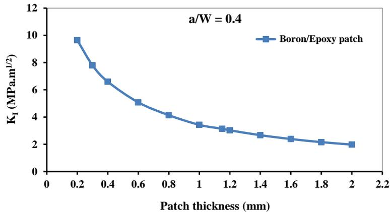
Fig. 6 Effect of double sided Boron/Epoxy composite patch thickness on  $K_I$
