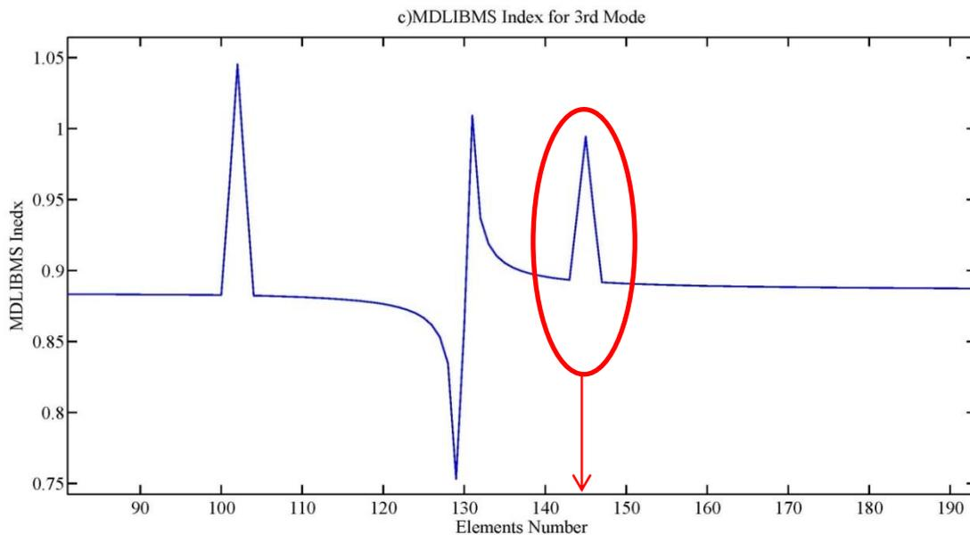
Fig. 10 3 spans steel bridge girder diagrams of MDLIBMS about element No.145 in third mode number
