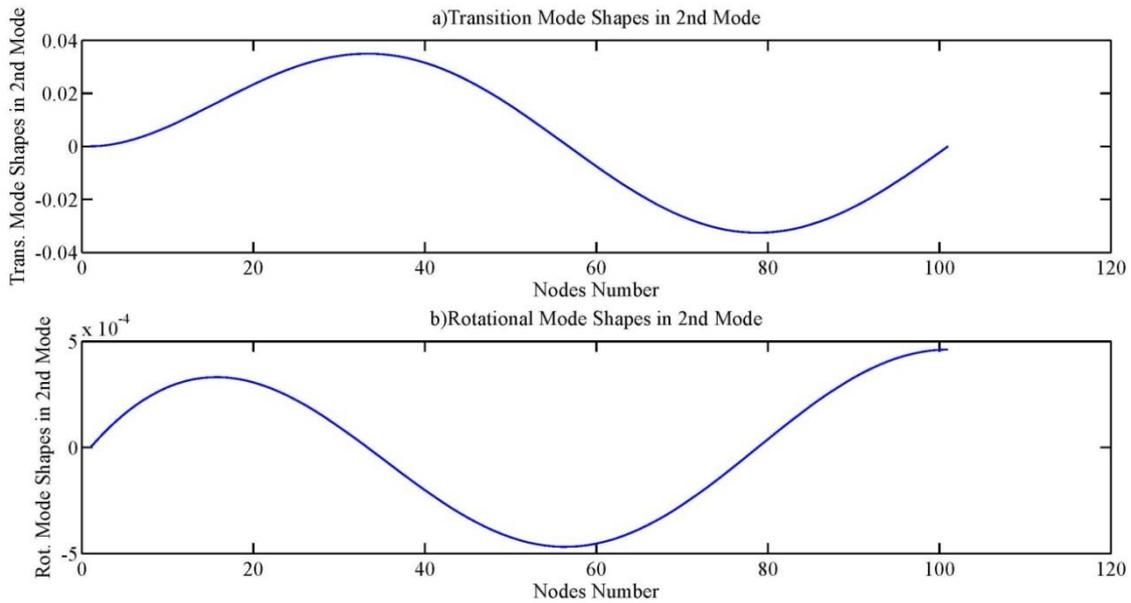
Fig. 6 100 elements fixed-pinned concrete beam diagrams (considering 5% noise) (a) Transverse mode shapes of the second mode number (b) Rotational mode shapes of the second mode number
