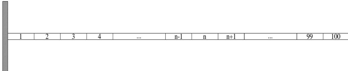
Fig. 2 A cantilever beam with 100 elements
