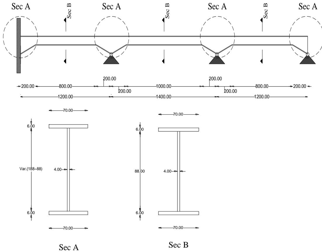
Fig. 7 A 3 spans steel bridge girder
