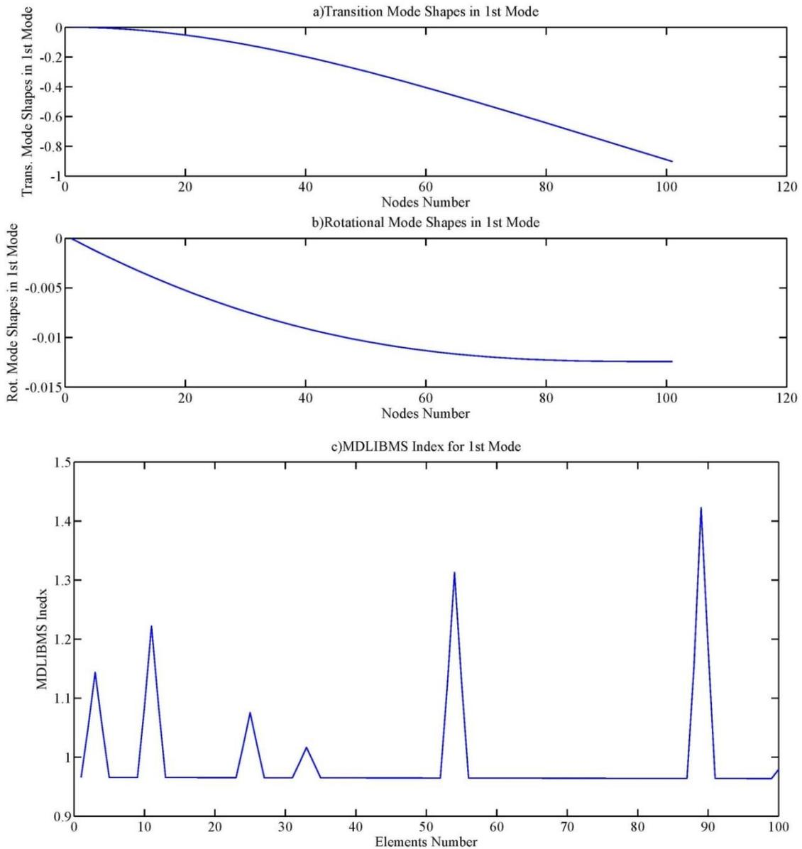
Fig. 3 100 elements cantilever beam diagrams (a) Transverse mode shapes of the first mode number (b) Rotational mode shapes of the first mode number (c) MDLIBMS criterion in the first mode
