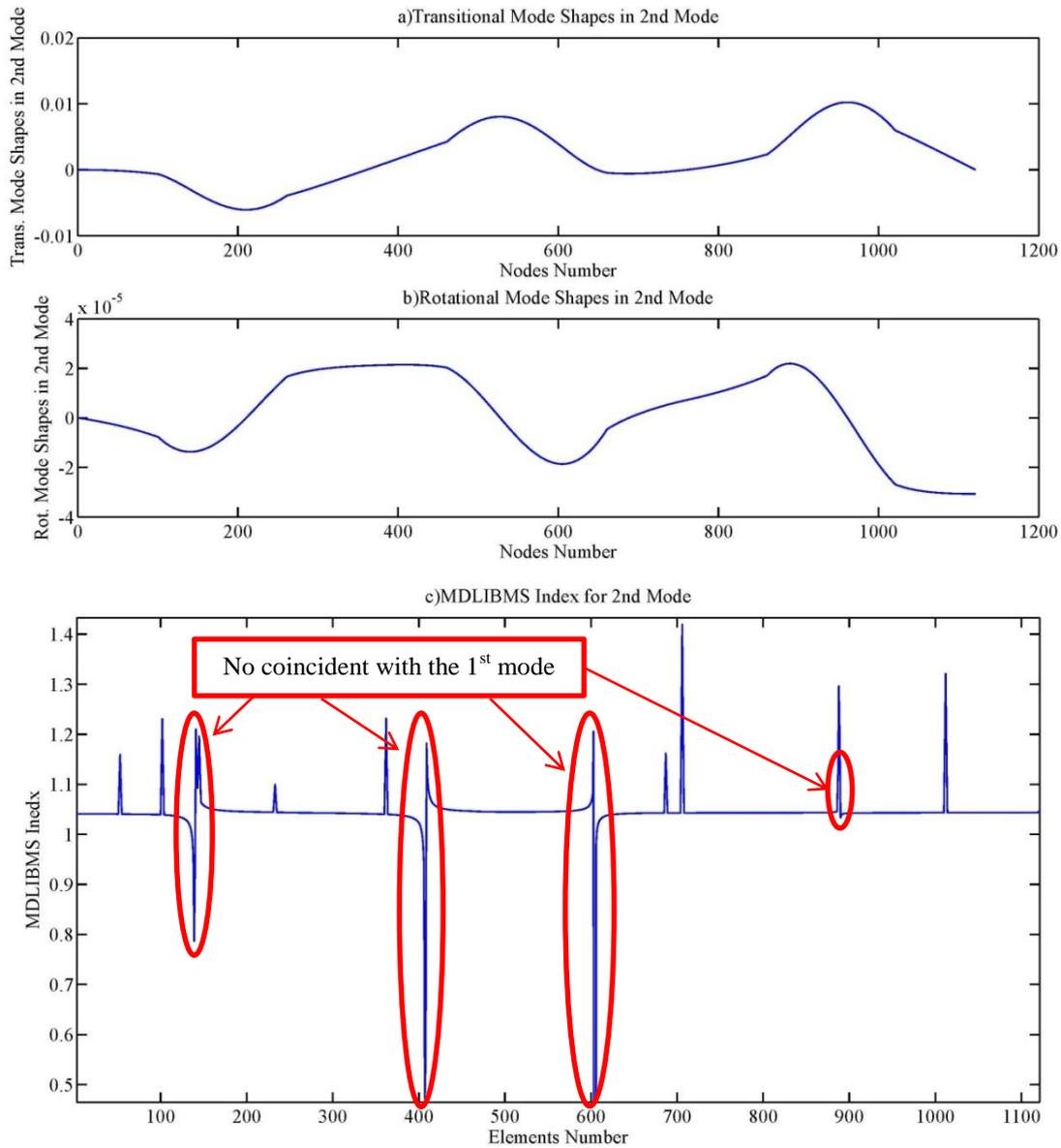
Fig. 9 3 spans steel bridge girder diagrams (considering 5% noise) (a) Transverse mode shapes of the second mode number (b) Rotational mode shapes of the second mode number (c) MDLIBMS criterion in the second mode (considering transverse modes only)
