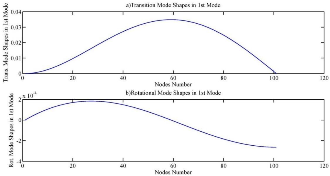
Fig. 5 100 elements fixed-pinned concrete beam diagrams (considering 5% noise) (a) Transverse mode shapes of the first mode number (b) Rotational mode shapes of the first mode number
