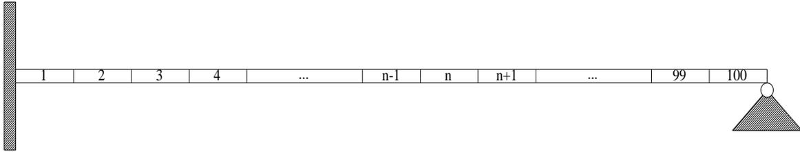
Fig. 4 A fixed-pinned concrete beam
