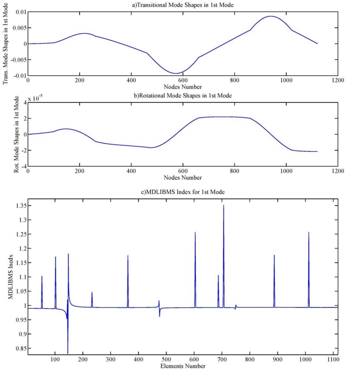
Fig. 8 3 spans steel bridge girder diagrams (considering 5% noise) (a) Transverse mode shapes of the first mode number (b) Rotational mode shapes of the first mode number (c) MDLIBMS criterion in the first mode (considering transverse modes only)
