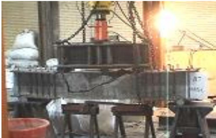
Fig. 4 The failure of beam B7
