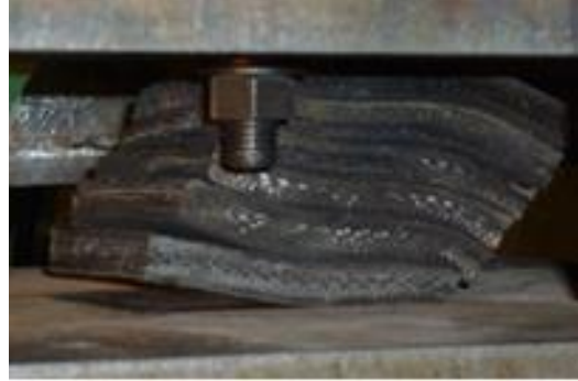
Fig. 18 Deformed state of layer-unbonded STRP-6 specimen under constant vertical pressure of 5 MPa at 103% shear strain
