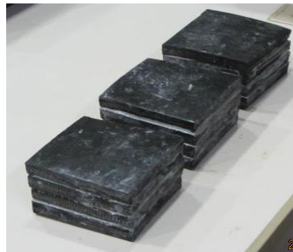
Fig. 6 Fully cured layers bonded samples
