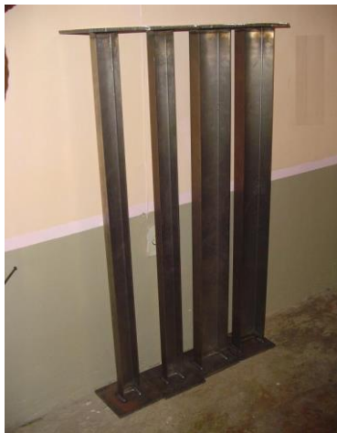
Fig. 8 View of the four channel columns used on the experimental tests (U110x55x1.2 and U65x35x1.5)
