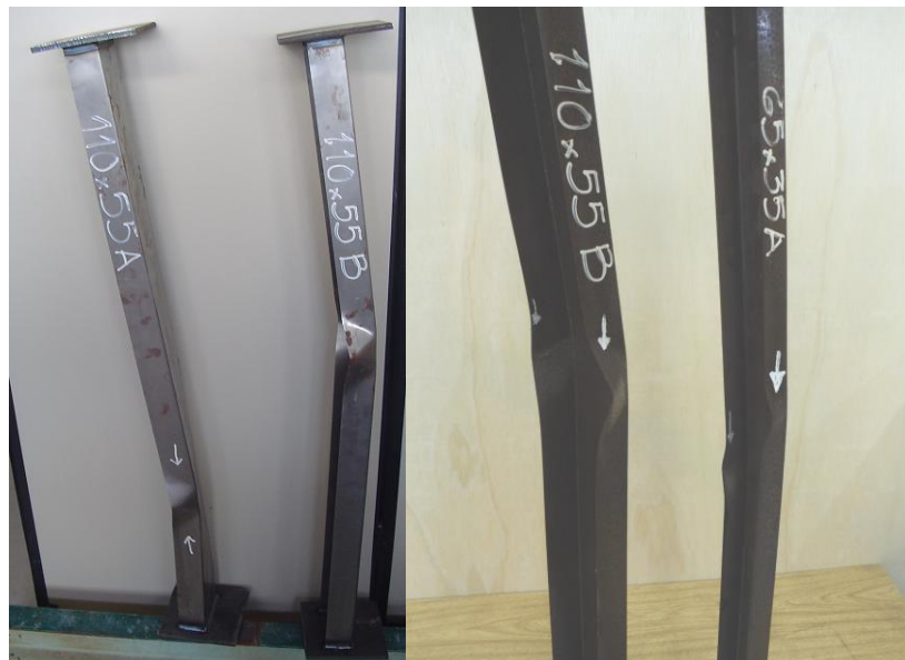
Fig. 10 Tested sections with local buckling deformation
