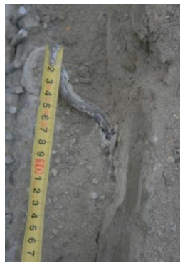
Fig. 22 Cut of jacketed specimen A-D m R c R j D b -1 after loading- dowel deformation
