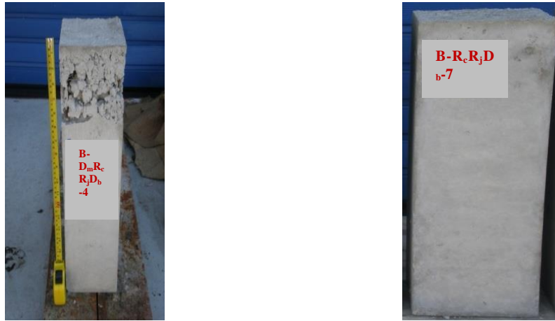
(a) Specimen with construction (initial) damages (b) Specimen without damages (B-R c R j D b -7)
