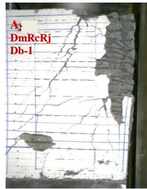
Fig. 23 Jacketed specimen A-D m R c R j D b -1 after failure of stirrups
