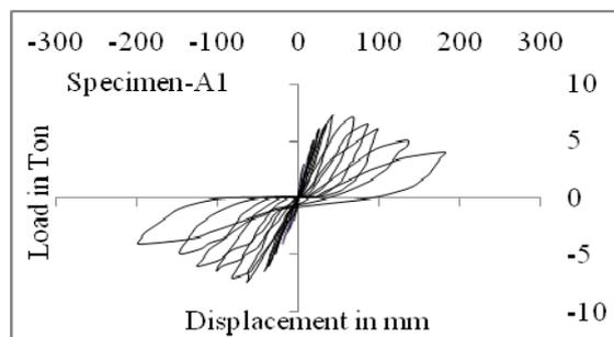
Fig. 9 Load Vs Displacement
