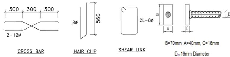
Fig. 8 Joint reinforcement bar and welded T-type headed bar
