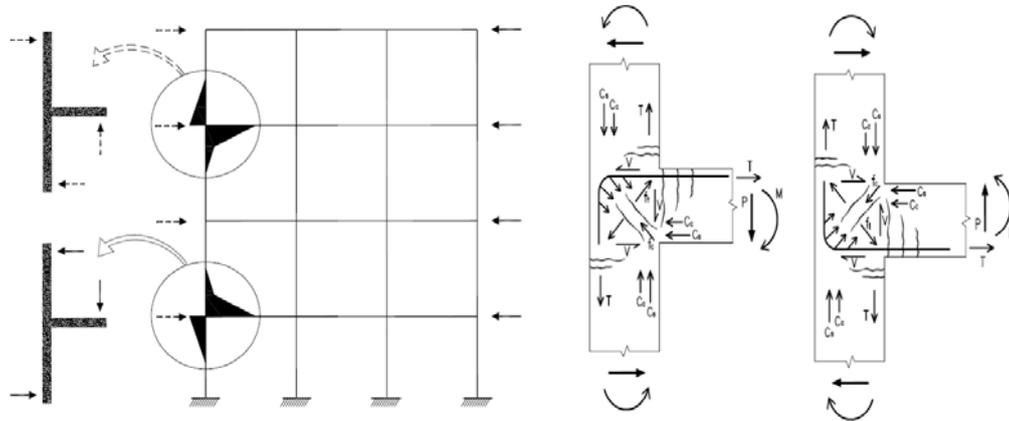
Fig. 2 Typical reinforced concrete frame and joint forces
