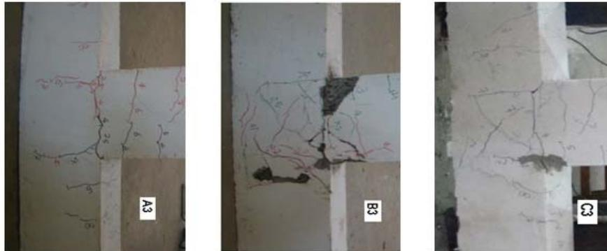
Fig. 34 Crack pattern of Group-IV (A3, B3, and C3)
