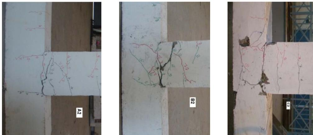
Fig. 33 Crack pattern of Group-II (A2, B2, C2)
