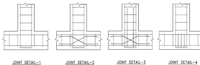
Fig. 7 Joint reinforcement arrangement
