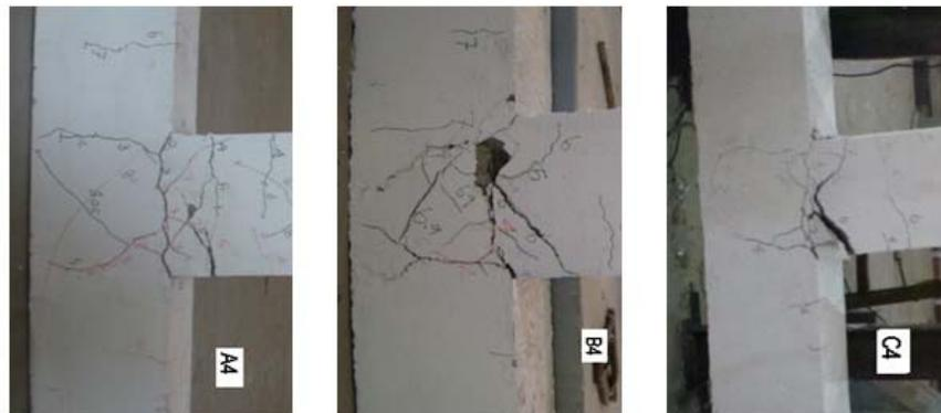
Fig. 35 Crack pattern of Group-IV (A4, B4, and C4)
