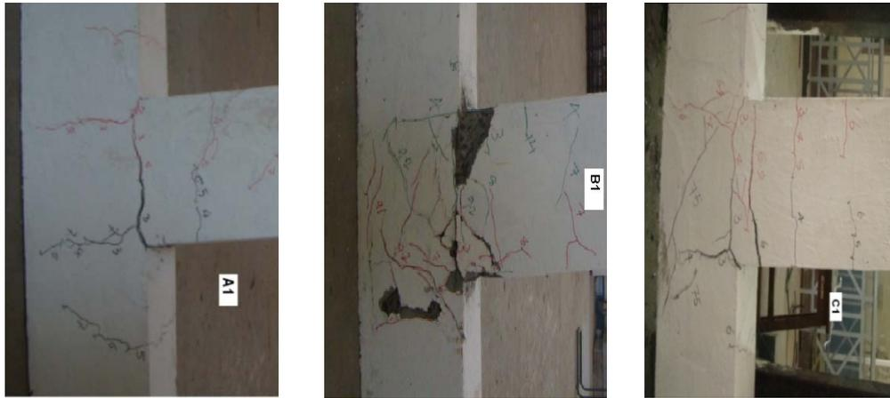
Fig. 32 Crack pattern of Group-I (A1, B1, and C1)
