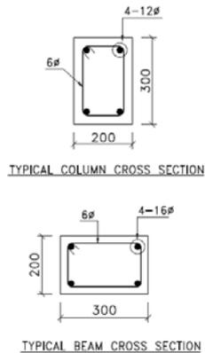
Fig. 3 Specimen size and bar details
