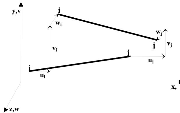
Fig. 1 Deformation of truss element  $ij$  in three dimensional space
