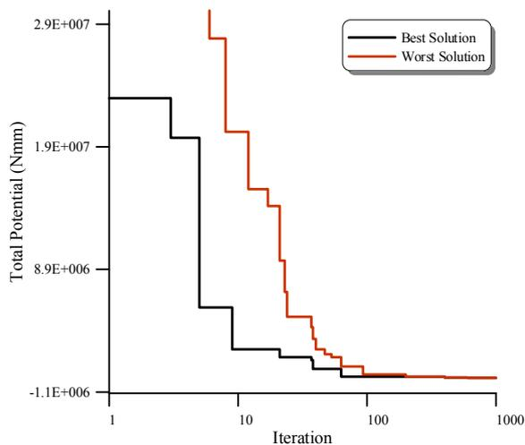
Fig. 4 Change of the total potential corresponding to best and worst solution vectors in the population as a function of the iterations for the 6-bar plane truss
