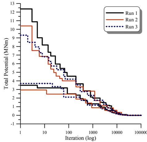
Fig. 8 Convergence of the best and worst vectors in three independent runs for the 25-bar space truss under Loading 1
