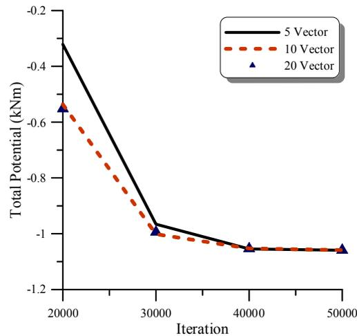
Fig. 6 Variation of total potential energy with respect to iterations and the number of vectors in the population for the 6-bar truss. The energy values are the averages of three independent runs
