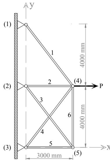
Fig. 3 6-bar plane truss
