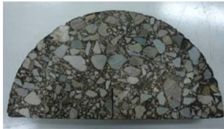
Fig. 4 An asphalt SCB speimen containing a thin crack
