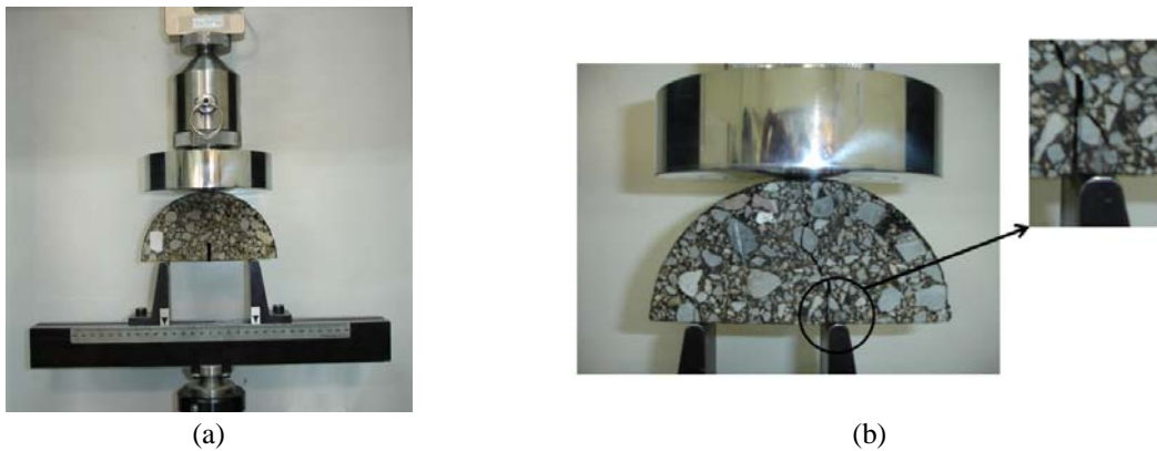
Fig. 6 Test configuration, (a) mode I fracture test, (b) unsuitable fixture setting for mode II fracture test
