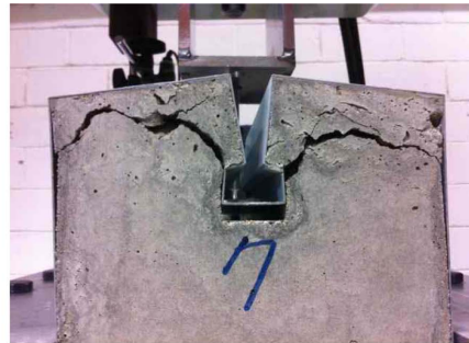
(b) Specimen type B (50-mm embedment)
