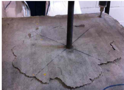
(c) Specimen type A (75-mm embedment)
