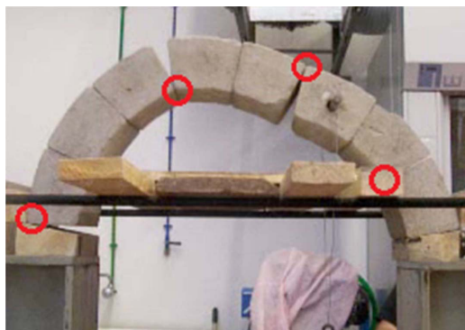
Fig. 2 Collapse mechanism of test B.2
