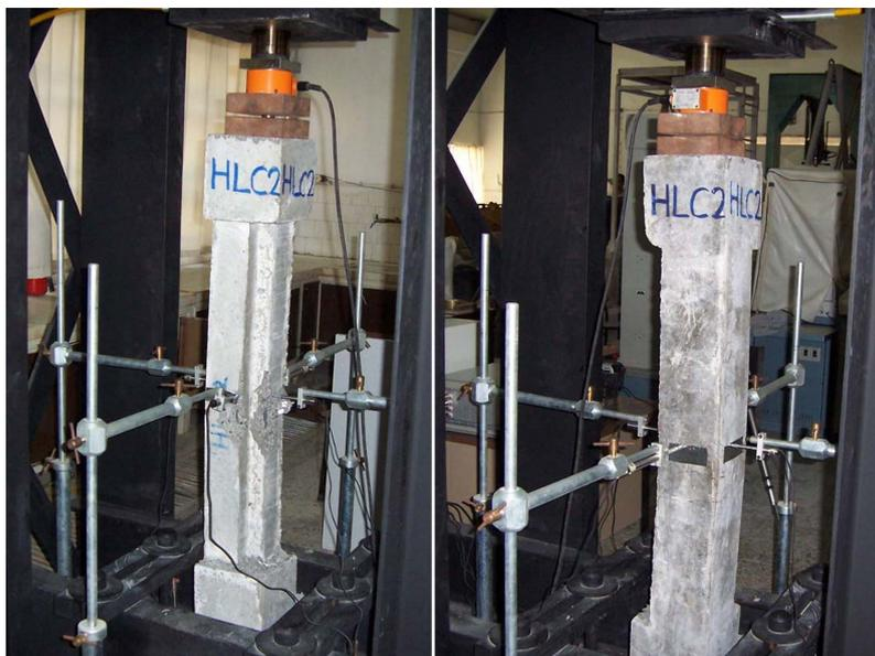
Fig. 3 Deflected shape of the column specimen HLC2
