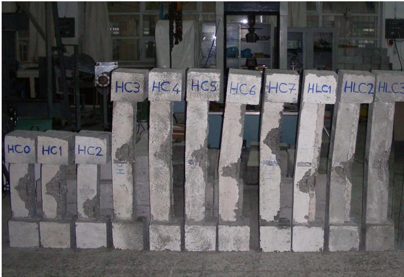
Fig. 5 Photo for all the column specimens after testing
