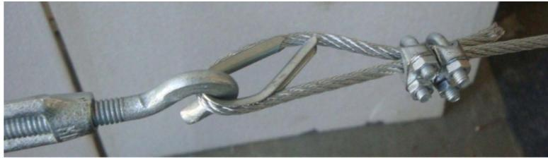
Fig. 14 Thimble anchoring failure: rotation due to clip fastening deficiency
