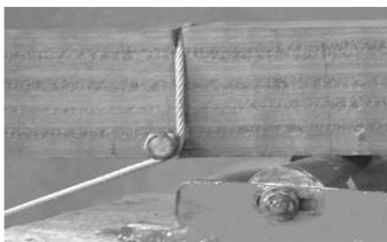
(a) Anchoring detail of the cable and beam
