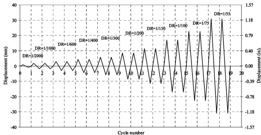
Fig. 5 Loading procedure
