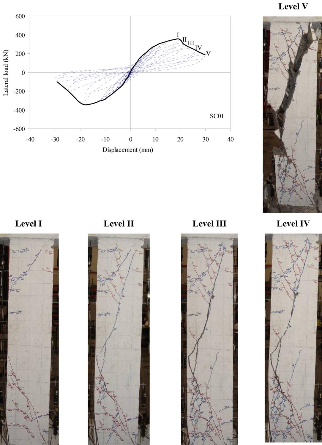
Fig. 7 Cracking patterns of tested specimen
