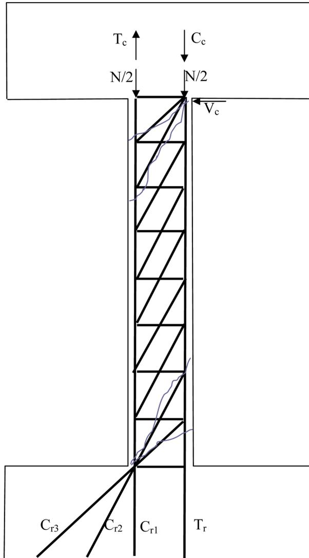
Fig. 1 Typical Strut-and-Tie Model for Lynn (2001), Sezen (2002)'s Specimens
