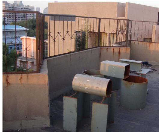
Fig. 1 Steel tube specimen on experiment site
