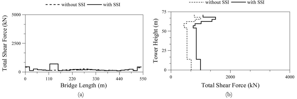
Fig. 11 Total shear forces of the bridge founded on firm soil; (a) deck, (b) tower
