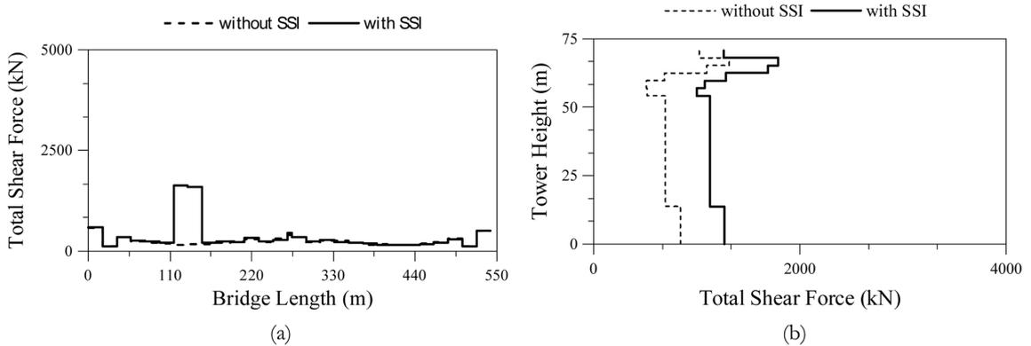
Fig. 10 Total shear forces of the bridge founded on medium soil; (a) deck, (b) tower
