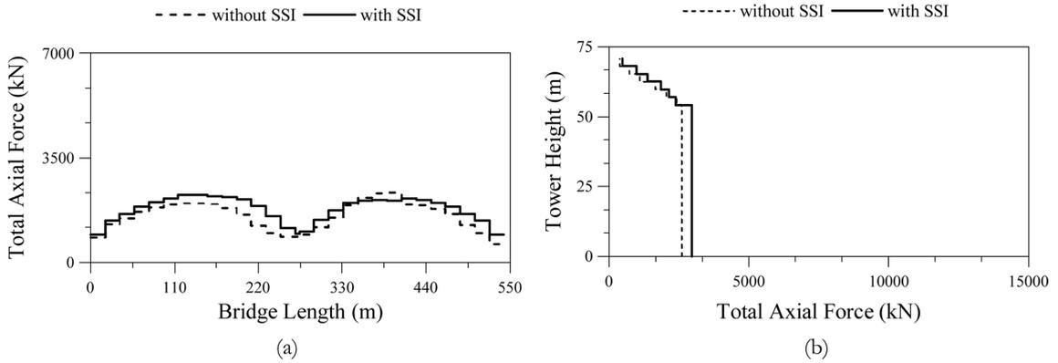
Fig. 8 Total axial forces of the bridge founded on firm soil; (a) deck, (b) tower
