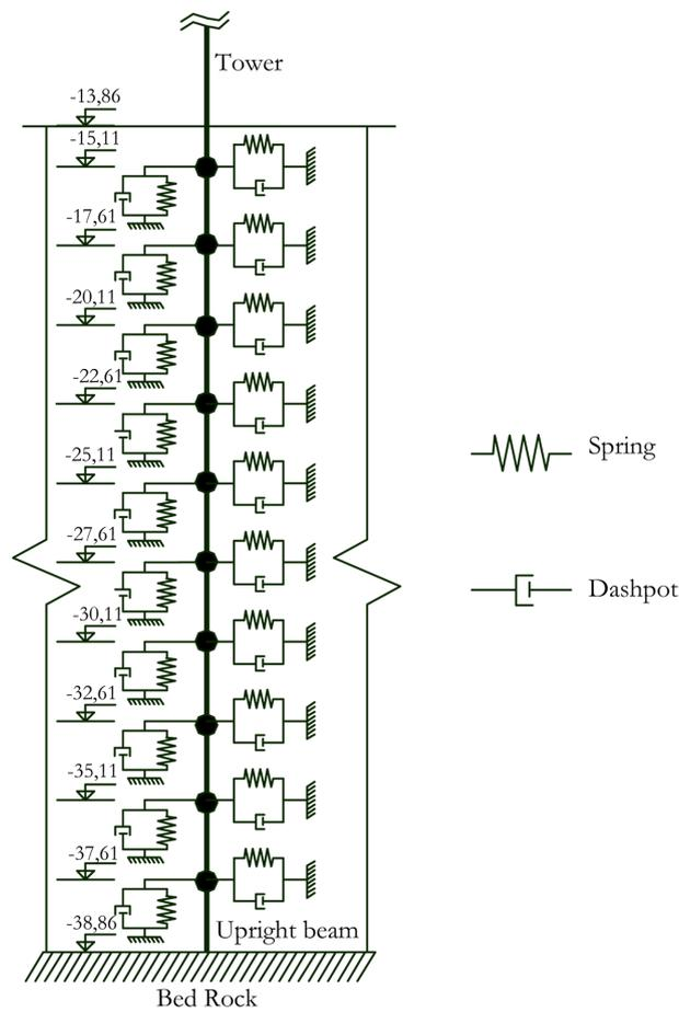
Fig. 5 Schematic of beam on Winkler foundation model in the layered soil strata
