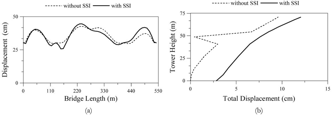
Fig. 15 Displacement of the bridge founded on soft soil; (a) deck, (b) tower
