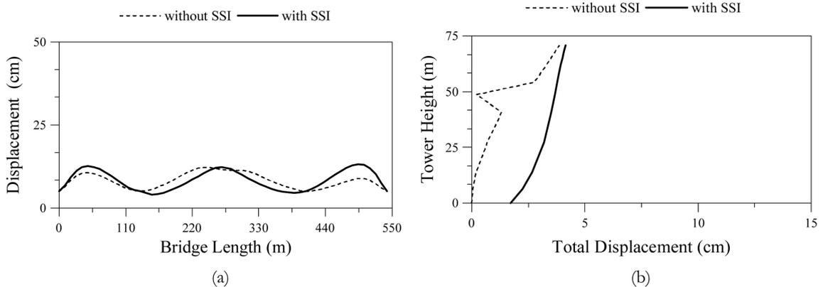
Fig. 17 Displacement of the bridge founded on firm soil; (a) deck, (b) tower
