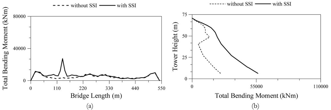
Fig. 13 Total bending moment of the bridge founded on medium soil; (a) deck, (b) tower
