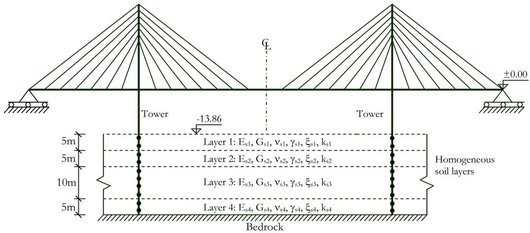
Fig. 4 Two dimensional finite element model of the soil-pile system
