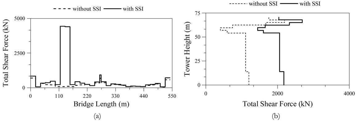
Fig. 9 Total shear forces of the bridge founded on soft soil; (a) deck, (b) tower
