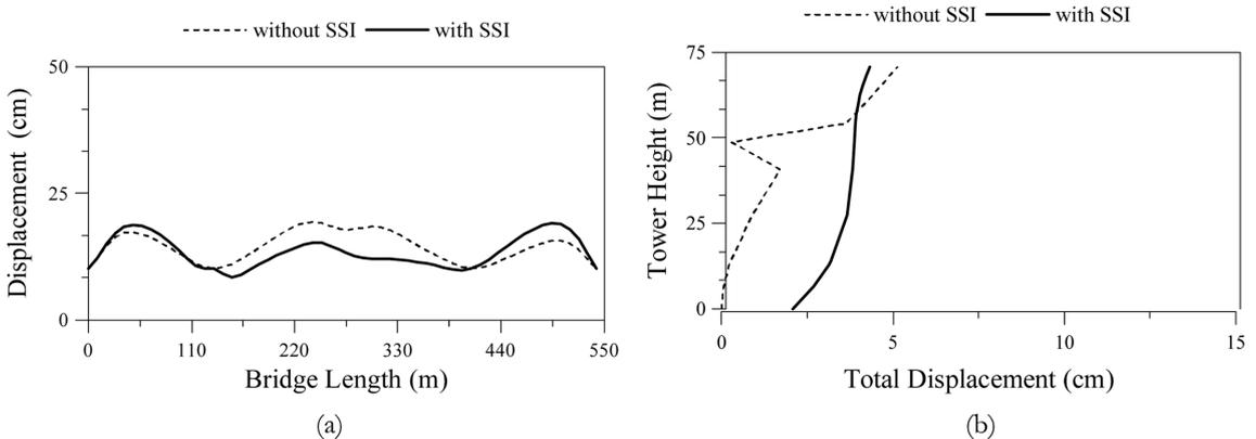
Fig. 16 Displacement of the bridge founded on medium soil; (a) deck, (b) tower
