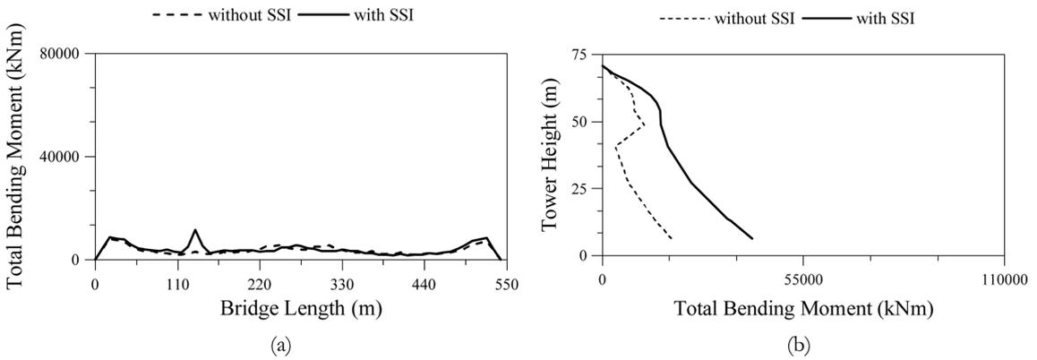
Fig. 14 Total bending moment of the bridge founded on firm soil; (a) deck, (b) tower
