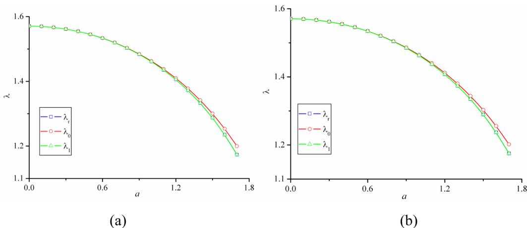
Fig. 2 The variations of the “reference” and approximate values of  $\lambda$  with the angle of rotation  $a$ , (a) for  $\rho = 0$  and (b) for  $\rho = 0.1$
