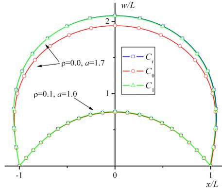
Fig. 5 Comparison of the “reference” and approximate post-buckling geometric configurations
