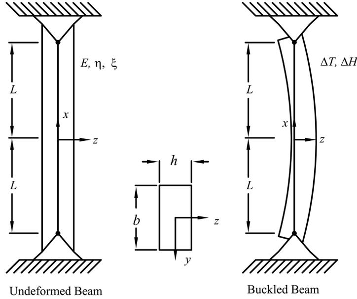
Fig. 1 Sketch of a simply supported beam subjected to hygrothermal loads
