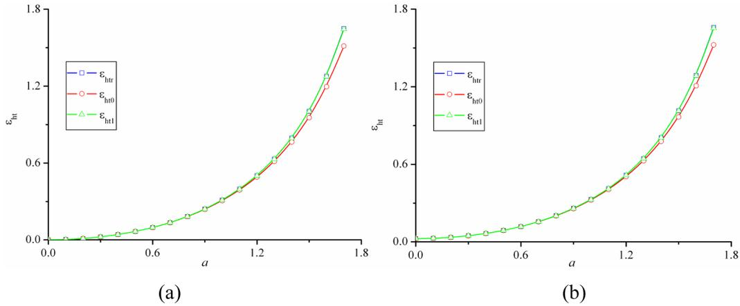
Fig. 3 The variations of the “reference” and approximate values of  $\varepsilon_{ht}$  with the angle of rotation  $a$ , (a) for  $\rho=0$  and (b) for  $\rho=0.1$
