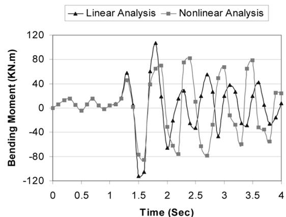
Fig. 6 One storey steel frame, comparison of beam bending moments in linear and nonlinear analysis
