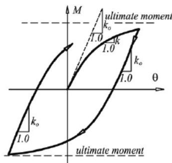
Fig. 1 Cyclic moment-rotation curve for a flexible connection
