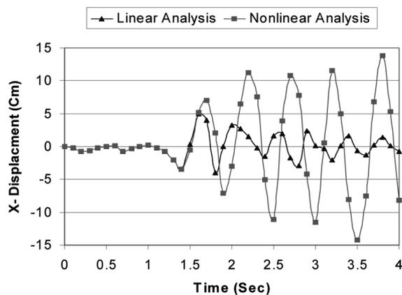
Fig. 5 One storey steel frame, comparison of drift in linear and nonlinear analysis
