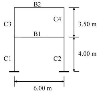
Fig. 7 Two storey steel frame
