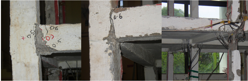
Fig. 20 Damage patterns observed at \text{PGA} = 0.6 \text{ g}
