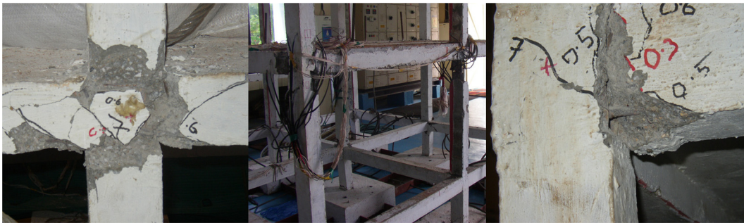
Fig. 21 Damage patterns observed at \text{PGA} = 0.7 \text{ g}
