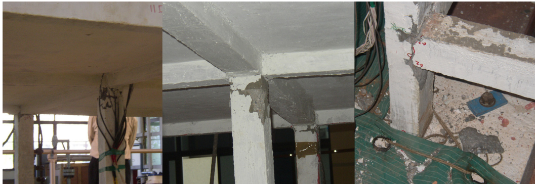
Fig. 19 Damage patterns observed at \text{PGA} = 0.5 \text{ g}
