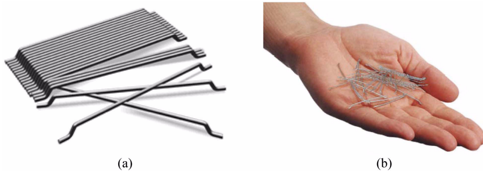
Fig. 1 Steel fibers (a) used in HPSFRC slabs (Dramix RC-80/60-BN), (b) used in SIFCON slabs (Dramix RL-45/30-BN) (Bekaert 2008)
