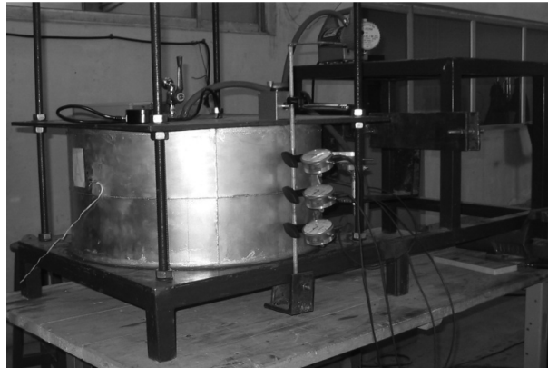
Fig. 3 View of test rig for cylindrical shell and gauges installation and specimens
