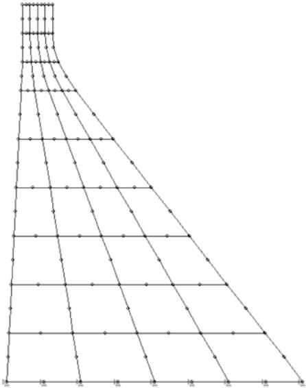
Fig. 2 Finite element discretization of Pine Flat dam
