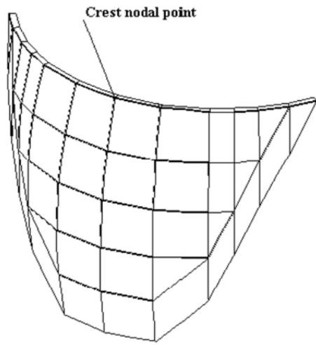
Fig. 3 Finite element mesh of Morrow Point dam
