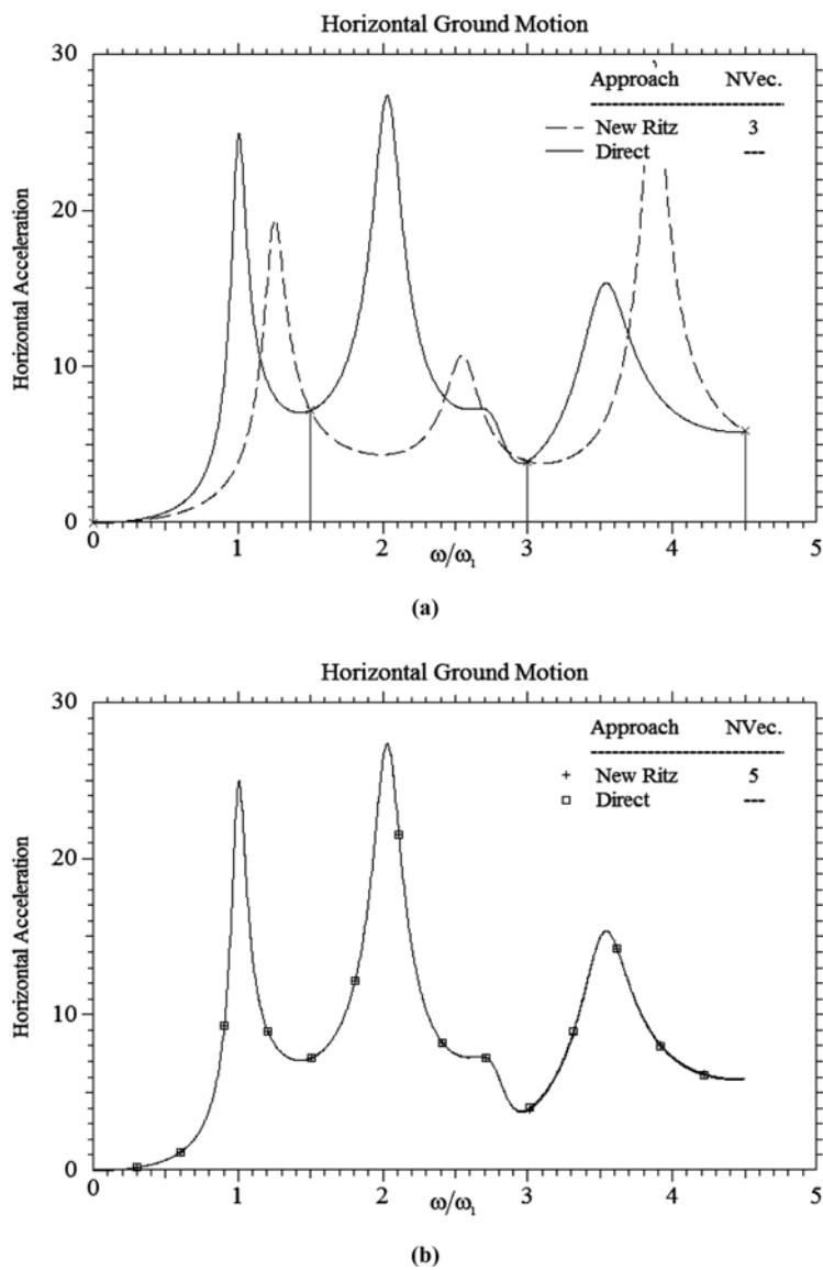
Fig. 4 Response of Model A based on new Ritz method (a) 3 Vectors, (b) 5 Vectors, (vertical lines shows the location of new Ritz vectors corresponding frequencies)
