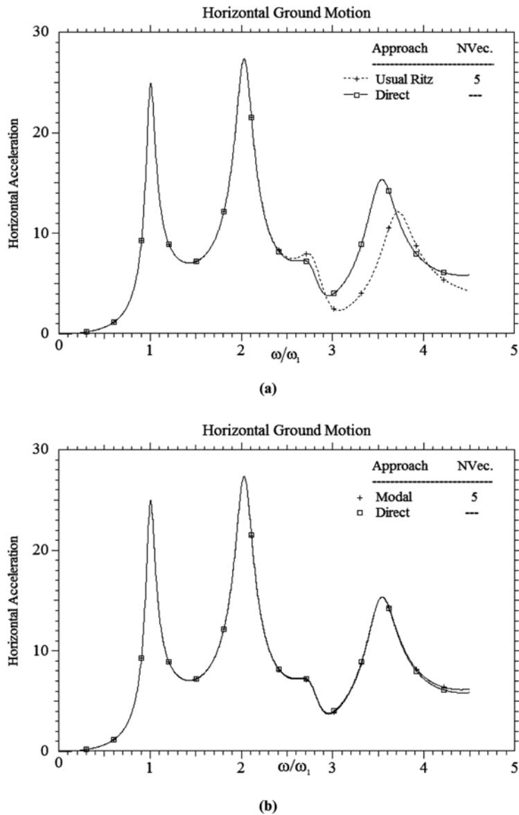
Fig. 5 Response of model A using usual Ritz and modal methods (horizontal excitation)
