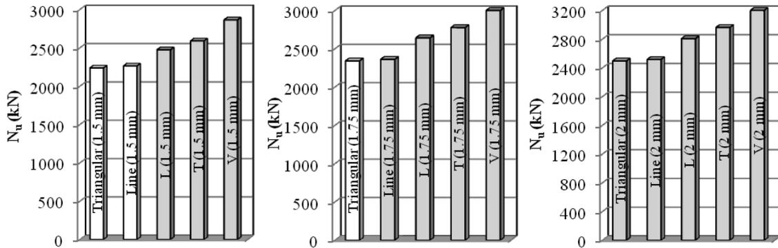
Fig. 27 Effect of shape of steel sheeting stiffeners on ultimate axial load capacity of the columns (2 on side stiffeners)
