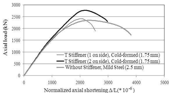
Fig. 17 Axial load-normalized axial shortening plots for columns with different number of T stiffeners (cold-formed 1.75 mm) and without stiffener (mild steel 2.5 mm)
