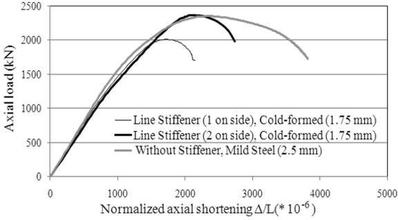
Fig. 19 Axial load-normalized axial shortening plots for columns with different number of Line stiffeners (cold-formed 1.75 mm) and without stiffener (mild steel 2.5 mm)
