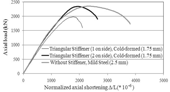
Fig. 20 Axial load-normalized axial shortening plots for columns with different number of Triangular stiffeners (cold-formed 1.75 mm) and without stiffener (mild steel 2.5 mm)
