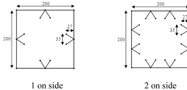
Fig. 6 Cross sections of the concrete-filled steel composite columns (V stiffeners & cold-formed steel sheets of 1.5, 1.75 & 2 mm) (All dimensions are in mm)
