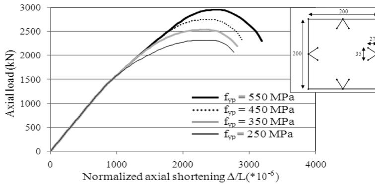
Fig. 31 Effect of yield stress  $f_{yp}$  of cold-formed steel sheet
