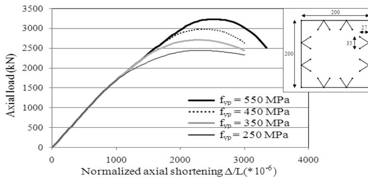
Fig. 32 Effect of yield stress  $f_{yp}$  of cold-formed steel sheet
