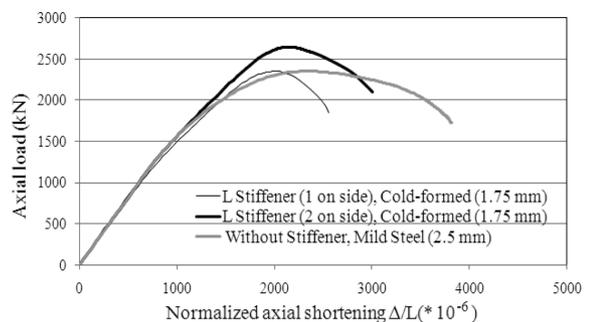
Fig. 18 Axial load-normalized axial shortening plots for columns with different number of L stiffeners (cold-formed 1.75 mm) and without stiffener (mild steel 2.5 mm)
