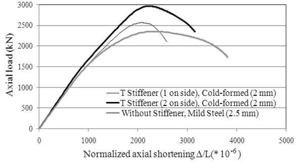
Fig. 22 Axial load-normalized axial shortening plots for columns with different number of T stiffeners (cold-formed 2 mm) and without stiffener (mild steel 2.5 mm)
