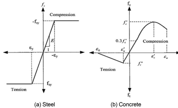
Fig. 3 Typical stress-strain curves for steel and concrete
