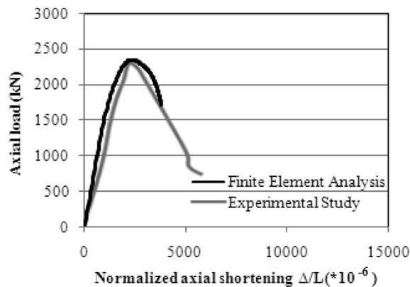
Fig. 5 Axial load-normalized axial shortening curves of the concrete-filled steel composite column (without stiffener, mild steel)
