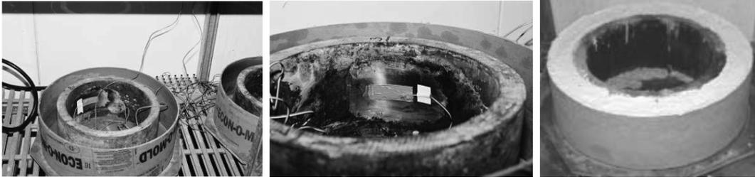
Fig. 3 Concrete ring framework and steel rings, the strain-gages position and the prepared ring specimen placed in environmental chamber
