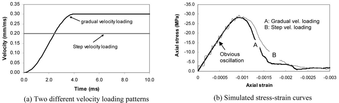
Fig. 4 Two different loading patterns and the resulting stress-strain responses
