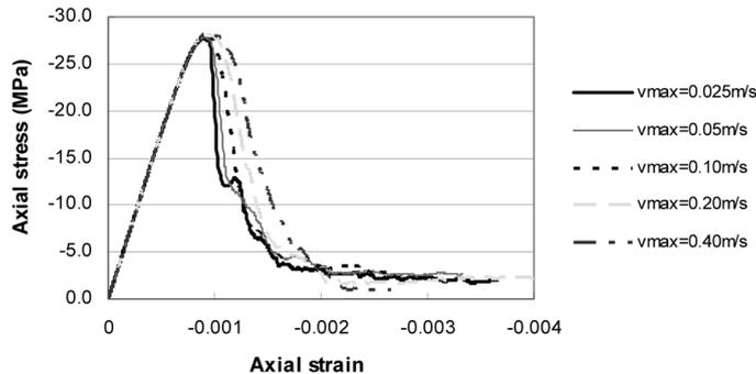
Fig. 5 Stress-strain responses obtained using different loading velocities
