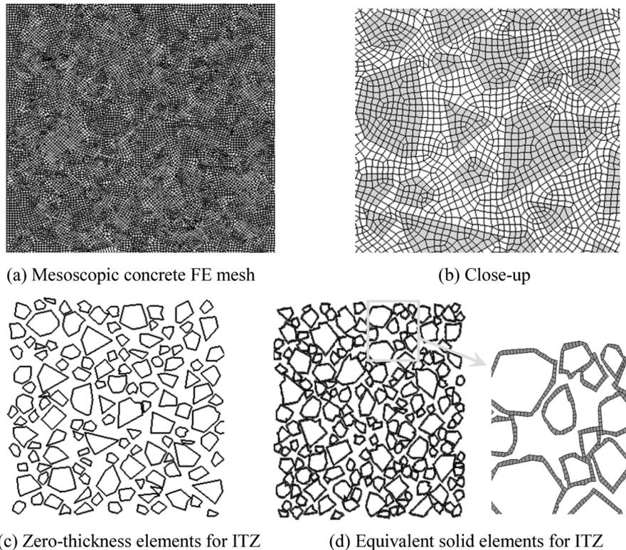
Fig. 3 Illustration of FE mesh for mesoscale model of concrete (Standard specimen size =  $150 \times 150$  mm)
