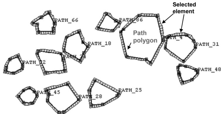
Fig. 7 Illustration of example paths and ITZ elements identified through these paths
