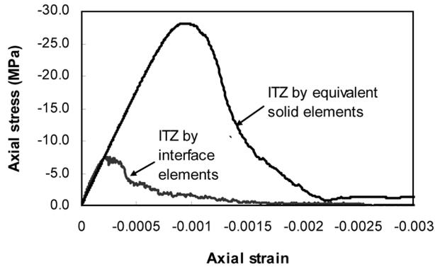
Fig. 9 Uniaxial compressive stress-strain relationships produced by mesoscale concrete model with two different ITZ modelling schemes
