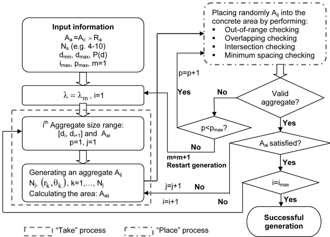
Fig. 2 Flowchart of generating random aggregate structure using take-and-place method
