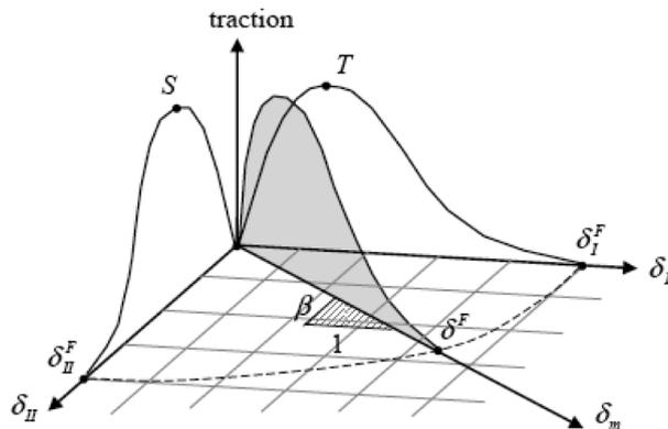
Fig. 8 Illustration of mix-mode constitutive law for cohesive elements (after LS-DYNA 2007)
