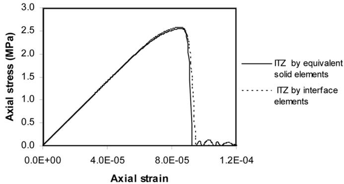
Fig. 10 Uniaxial tensile stress-strain relationships produced by mesoscale model with two different ITZ modelling schemes
