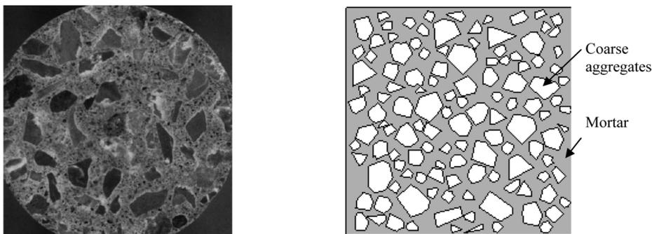
(a) Physical sample (after Grote *et al.* 2001) (b) Numerically generated model (not to match with (a))
