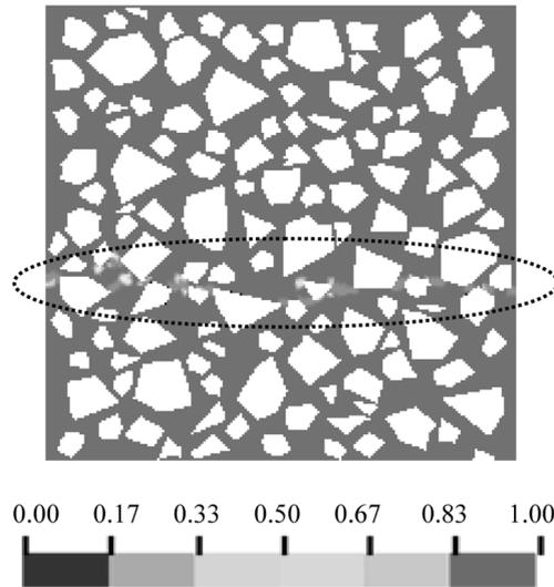
Fig. 11 Simulated fracture pattern of concrete under uniaxial tension using interface elements for ITZ (Note: the colour scale indicates damage with 1.0 being total damage)
