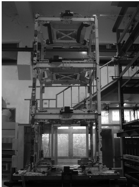
Fig. 1 A benchmark problem of a three-story 30% scaled steel structure
