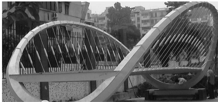
Fig. 2 Scaled model of special-shape arch bridge for self-balance
