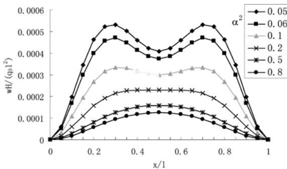
Fig. 3 Displacement under the position of a concentrated load ( $\lambda^2 = 400$ )
