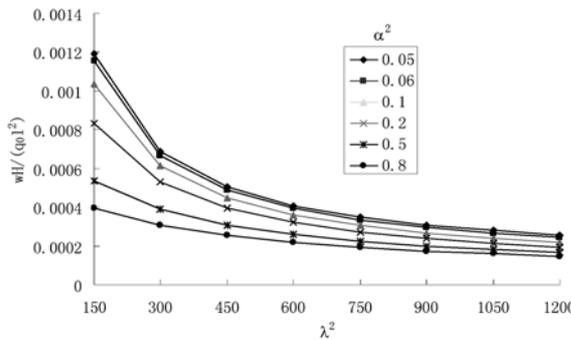
Fig. 7 Maximum displacement under distributed load ( $q = 0.1q_0$ )
