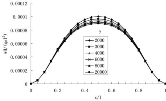
Fig. 5 Displacement under the position of a concentrated load ( $\lambda^2 = 770$ ,  $\alpha^2 = 0.77$ )
