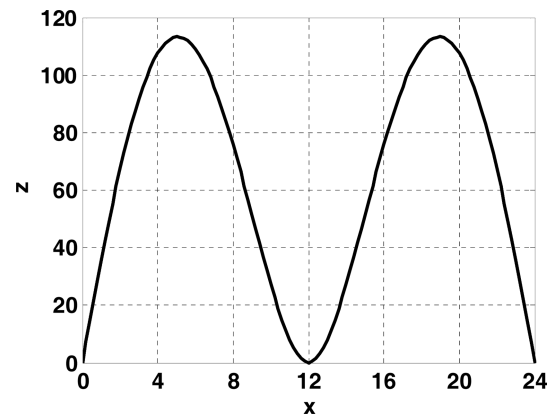
Fig. 11 Deflected shape due to udl in both spans
