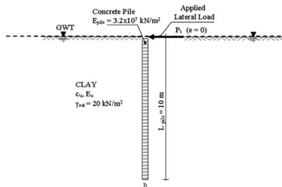
Fig. 1 Schematic view of soil-pile model used in the analysis
