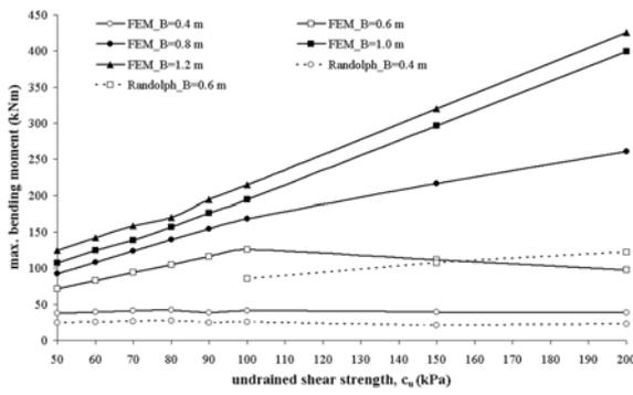
Fig. 5 Variation of the maximum bending moment with undrained shear strength and pile diameter
