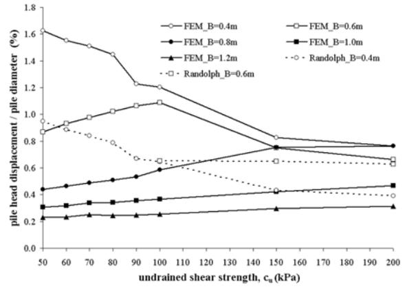
Fig. 6 Dimensionless pile head displacement parameter as a function of undrained shear strength and pile diameter
