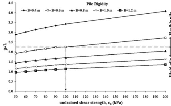
Fig. 4 Pile diameter-pile rigidity relationship at various undrained shear strength values
