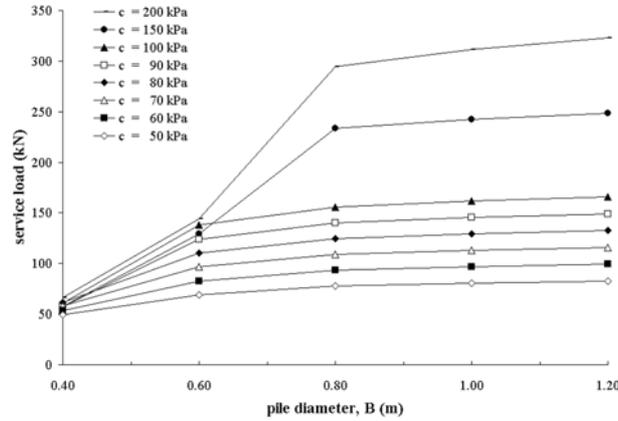
Fig. 2 Service loads on piles
