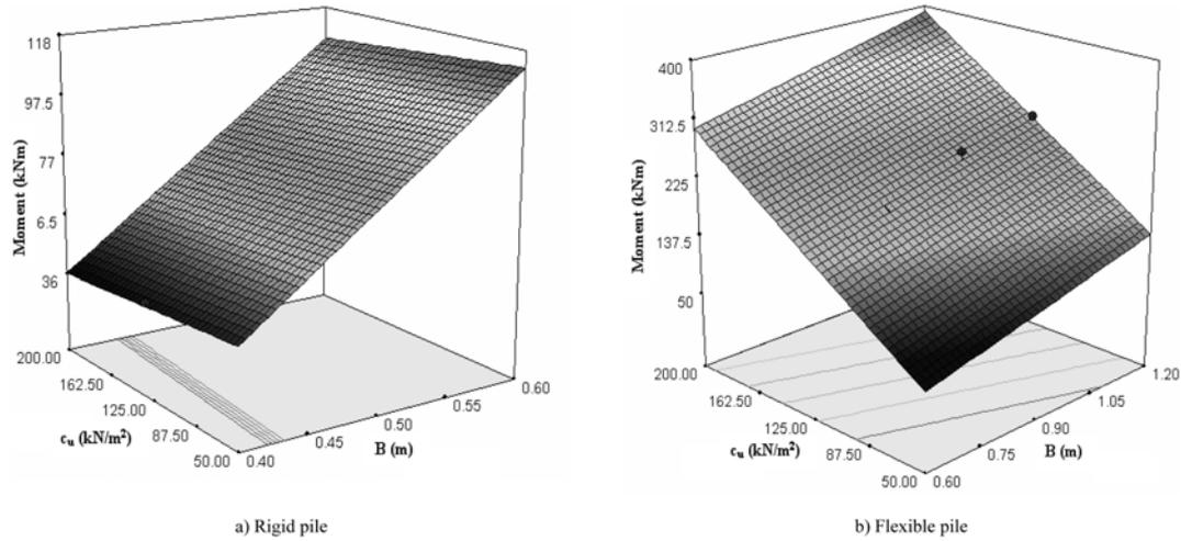
Fig. 7 Variation of the estimated maximum bending moment with undrained shear strength and pile diameter
