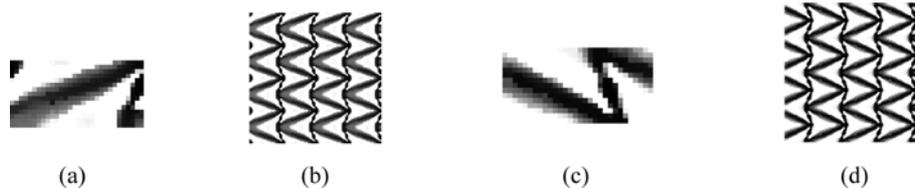
Fig. 2 Microstructure with negative poisson's ratio (a) the upper half base cell by 2 norm optimization model, (b) 4×4 repeating unit cells of a, (c) the upper half base cell by cross entropy optimization model, (d) 4×4 repeating unit cells of c
