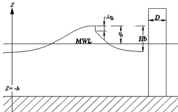
Fig. 1 A typical model of wave loads
