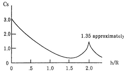
Fig. 2  $C_s$  as a function of relative submergence
