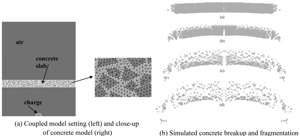
Fig. 6 Simulation of concrete break-up under internal explosion with mesoscale model
