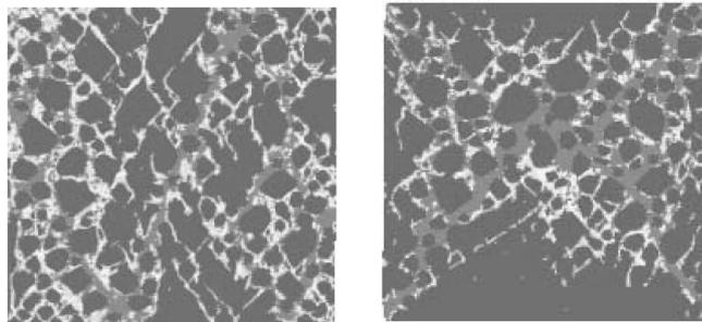
(b) Computed damage patterns under quasi-static compression without (left) and with (right) loading face friction
