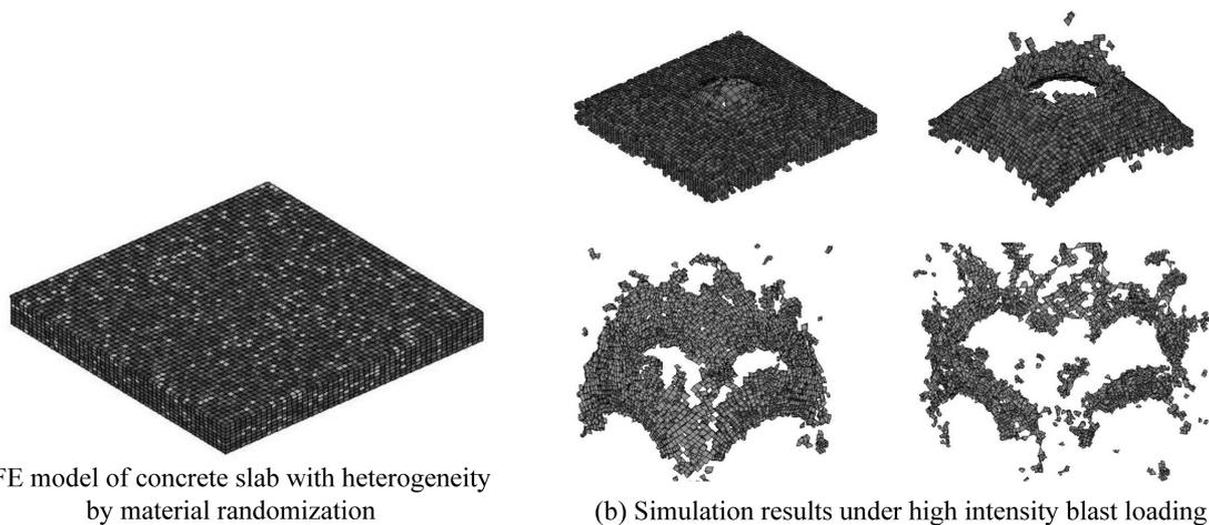
(a) FE model of concrete slab with heterogeneity by material randomization
