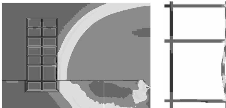
Fig. 1 A finite element model for structural response to combined air blast and ground shock
