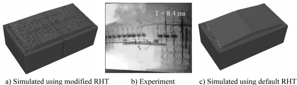
Fig. 8 Crack patterns of an RC slab: simulated vs. experimental
