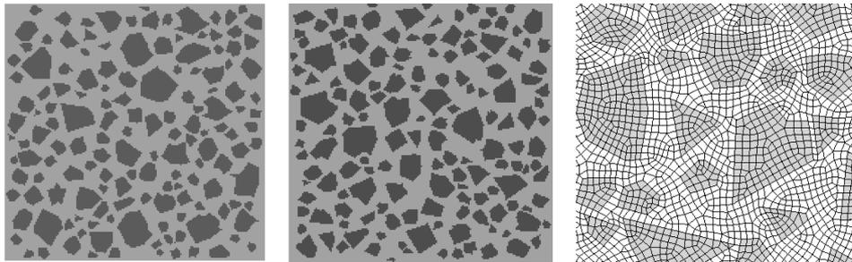
(a) Typical generated mesoscale geometry and FE mesh for concrete
