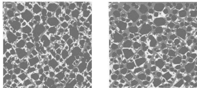
(c) Computed damage patterns under high rate loading (left =  $10 \text{ s}^{-1}$ ; right =  $100 \text{ s}^{-1}$ )
