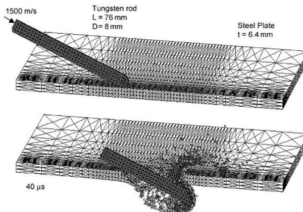
Fig. 3 Impact of a tungsten rod onto a steel plate (After Johnson and Stryk 2003)
