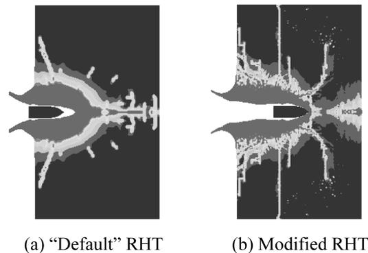
Fig. 9 Simulated penetration of steel projectile in 800 mm-thick concrete target
