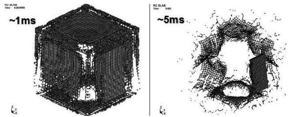
Fig. 11 Simulated break-up of concrete box structure under large internal explosion
