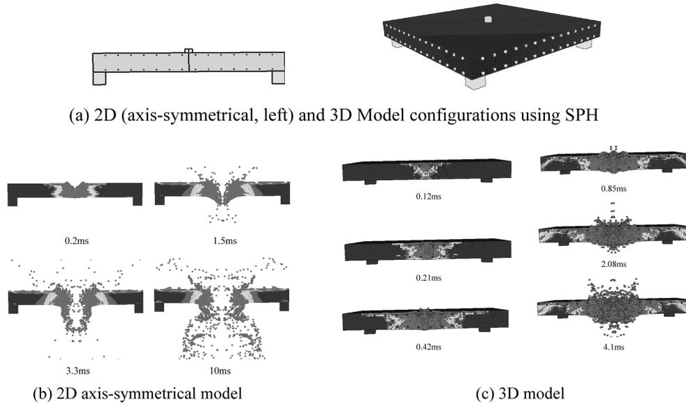
Fig. 10 Modelling of RC slab under contact explosion using SPH
