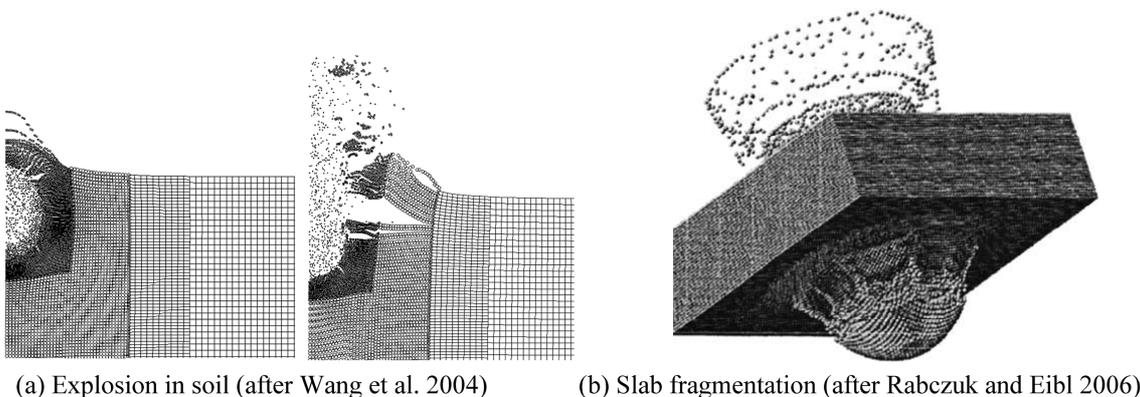
Fig. 2 SPH models for simulation of cratering and fragmentation
