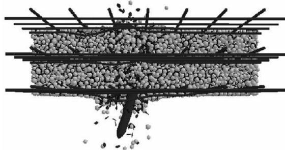
Fig. 4 Simulation of penetration using LDPM (After Cusatis and Pelessone 2006)
