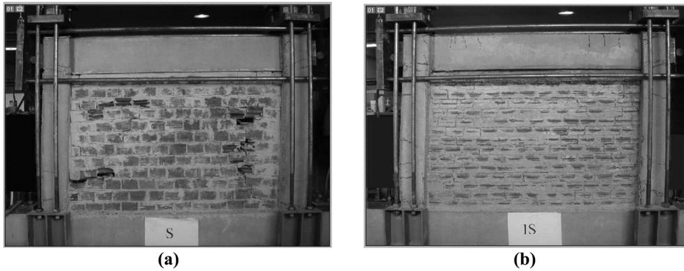
Fig. 5 Failure mechanisms of the solid infill: (a) compression failure of the weak solid infill, (b) shear-sliding failure of the strong solid infill
