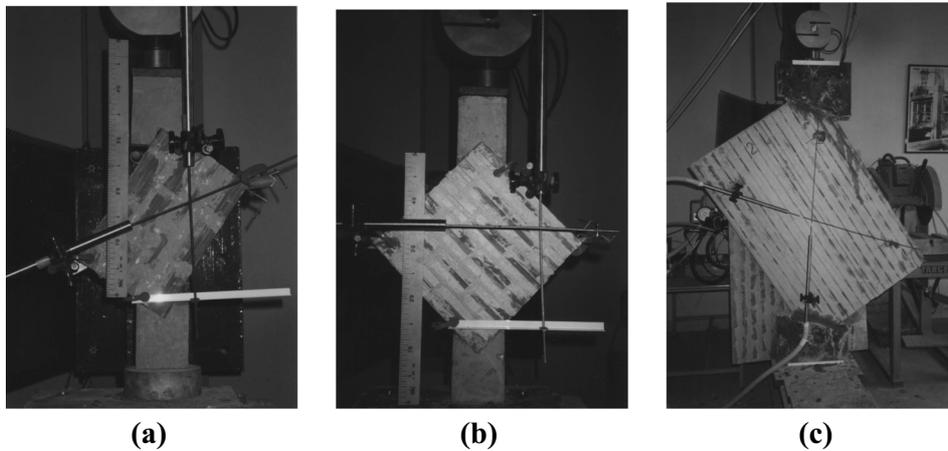
Fig. 2 The diagonal compression tests: (a), (b) masonry panels with various length  $L_i$  to height  $H_i$  ratios, (c) full size masonry panels
