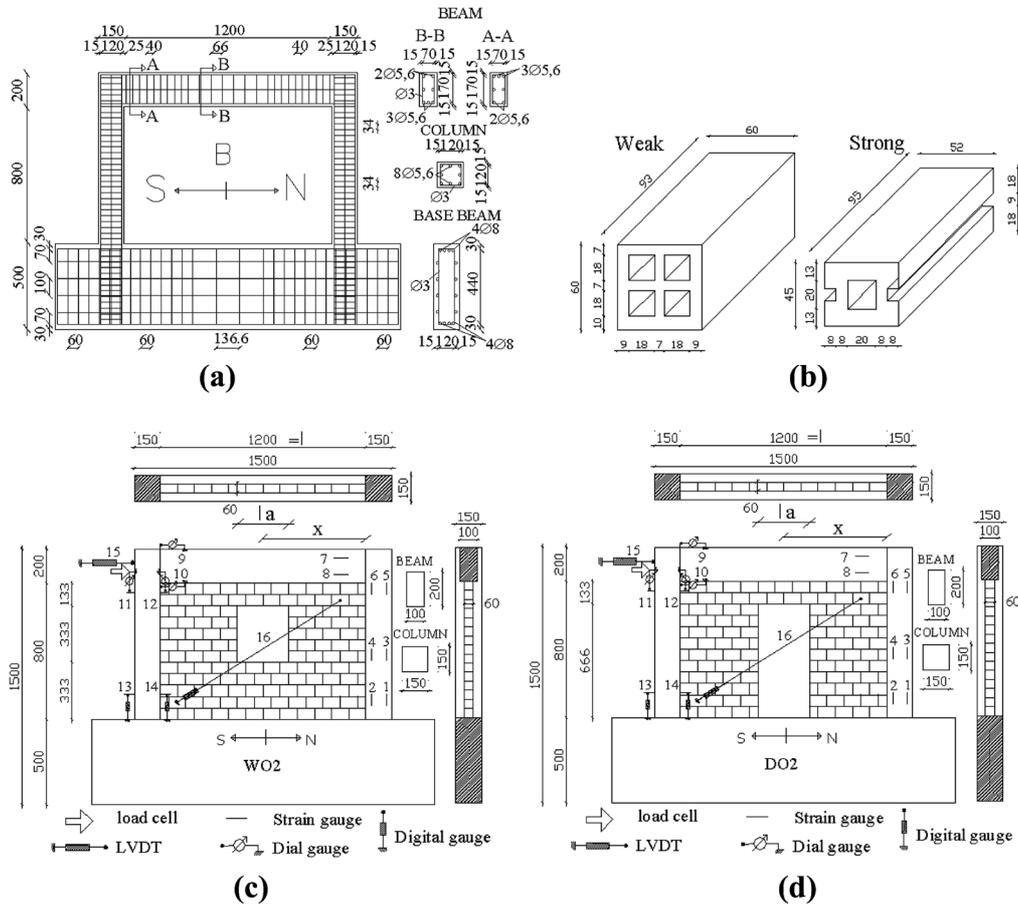
Fig. 1 Description of infilled frame specimens and instrumentation (mm): (a) reinforcement detailing of the R/C frame model, (b) weak and strong brick units, (c) specimen with window opening and instrumentation, (d) specimen with door opening and instrumentation
