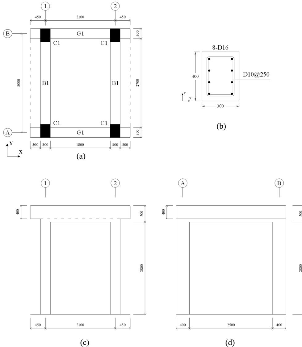
Fig. 8 Layout of simple reinforced concrete structure: (a) top view, (b) cross section of column C1, (c) front view and (d) side view
