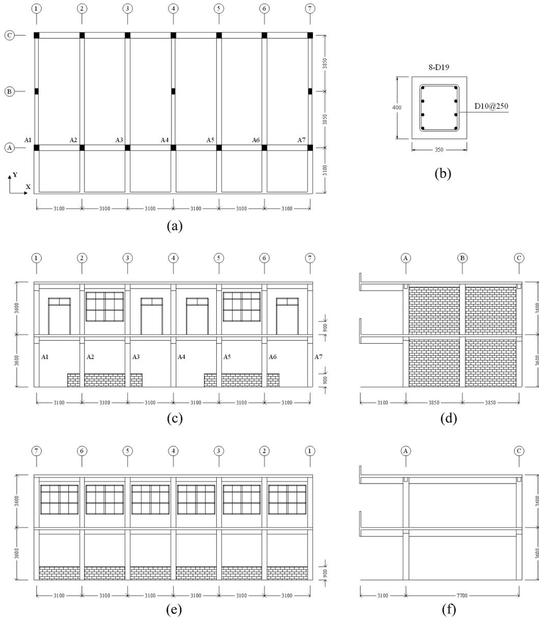
Fig. 13 Layout of Reupu Elementary School building: (a) typical top view of the 1<sup>st</sup> and 2<sup>nd</sup> floor, (b) cross section of columns A1 through A7, (c) front view, (d) sectional view of portals 1, 4, and 7, (e) back view and (f) sectional view of portals 2, 3, 5, and 6.
