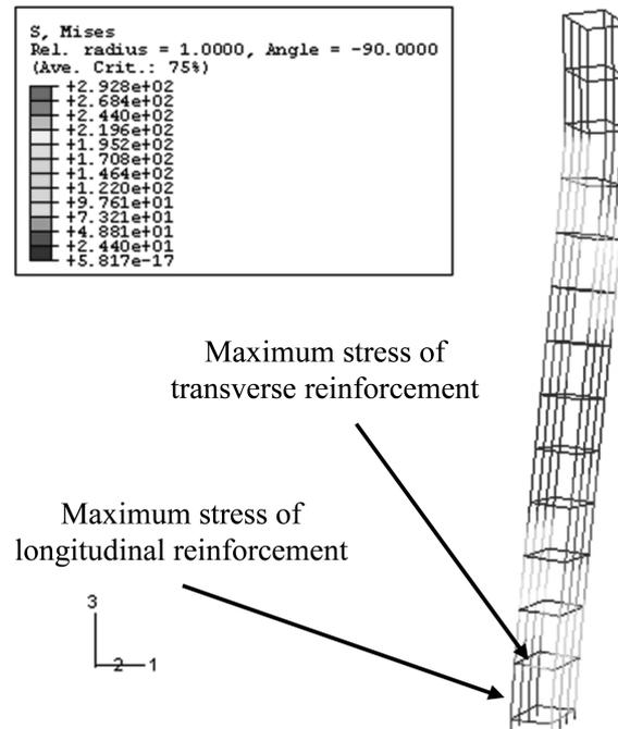
Fig. 12 The RCM simulated response of the steel rebar within a simple reinforced concrete column, as found in the experimental structure
