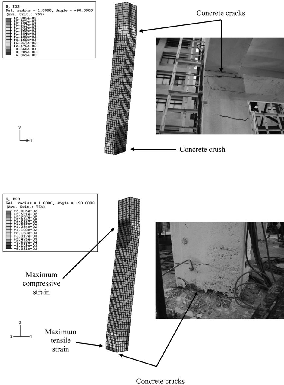
Fig. 11 Comparison of the RCM simulated response and photographs of an actual experiment for the column of a simple reinforced concrete structure
