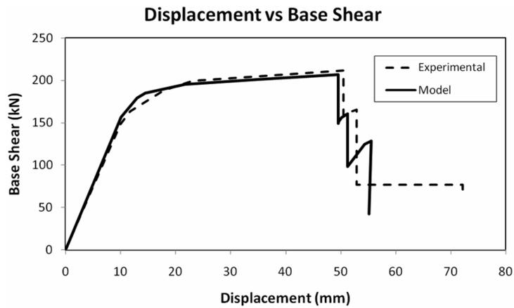
Fig. 10 Comparison of capacity curves for the analytical model and experimental results for a simple reinforced concrete structure
