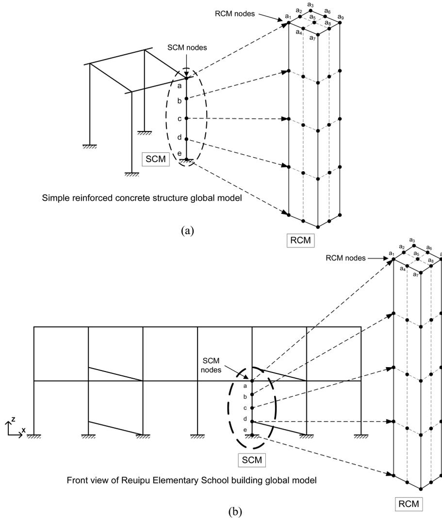
Fig. 7 Representations of two-level hierarchical models for (a) simple reinforced concrete structure and (b) Reuipu Elementary School building
