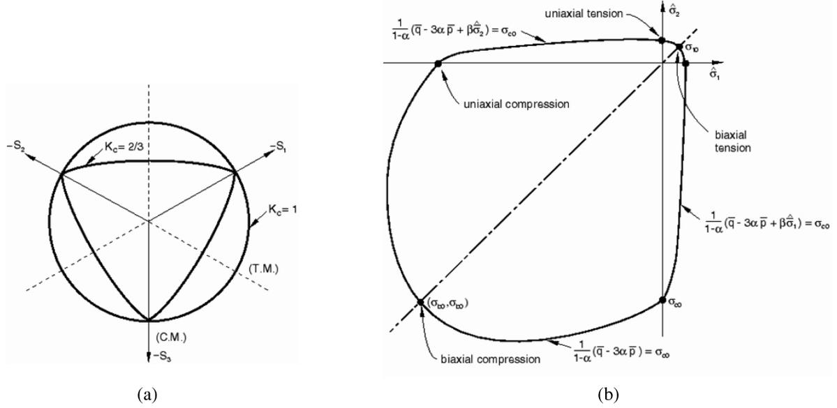
Fig. 3 Yield surfaces in: (a) the deviatoric plane, corresponding to different values of  $K_c$  and (b) the plane stress (ABAQUS 2004).
