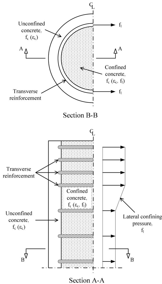
Fig. 4 Confined concrete associated with lateral confining pressure in the column component
