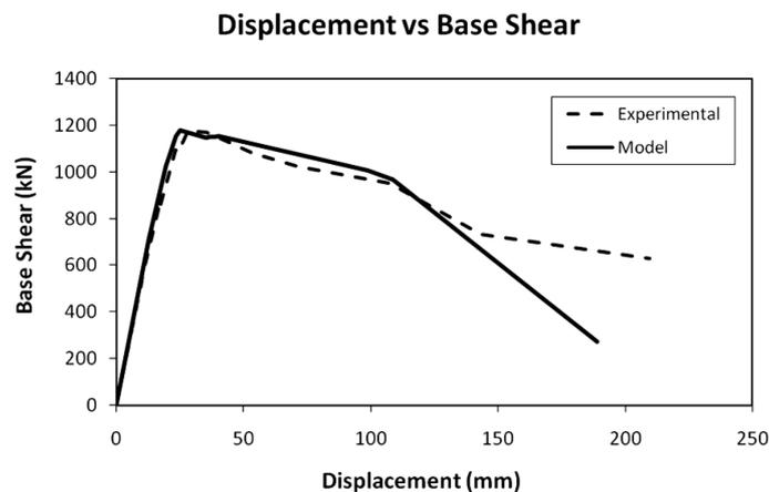
Fig. 15 Comparison of capacity curves for the analytical model and experimental results for Reuipu Elementary School building
