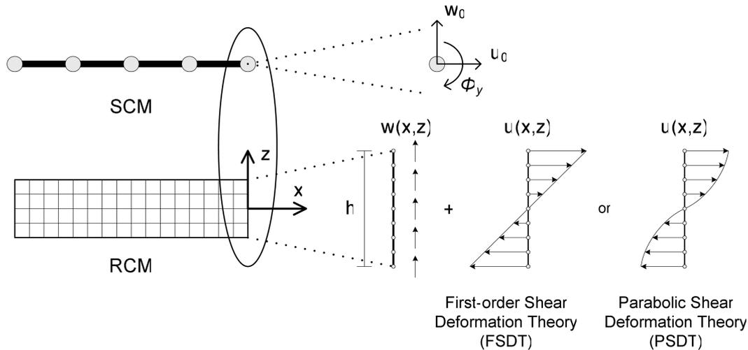
Fig. 5 The extracting and translating mechanism of nodal displacement from SCM to RCM
