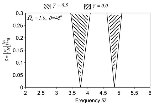
Fig. 2 The lowest unstable region of a rotating beam system with and without a crack
