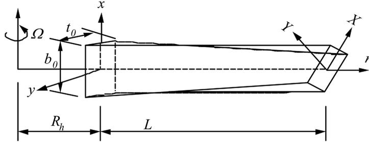
Fig. 1 Geometry of the rotating taper pre-twisted beam
