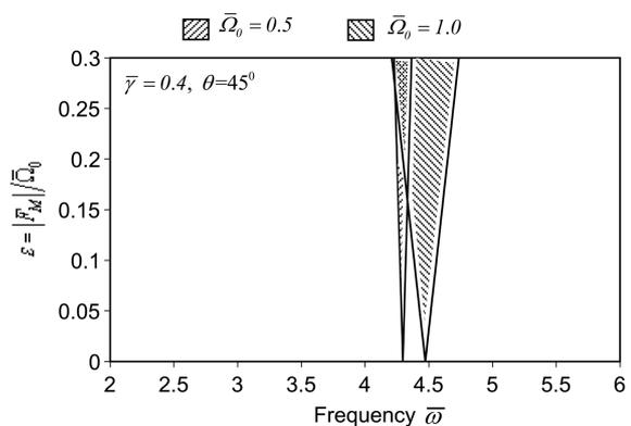
Fig. 3 The lowest unstable region of the beam system with different rotating speed
