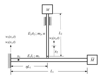
Fig. 1 Vibrational system under study: A cantilevered beam with a tip mass and in-span an axially vibrating visco-elastic rod with a tip mass
