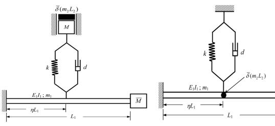
Fig. 3 Simplified representation of the vibrational system in Fig. 1
