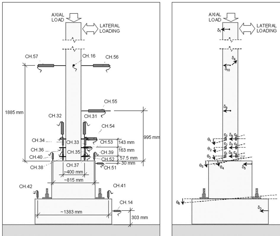
Fig. 4 Instrumentation for displacements and curvatures
