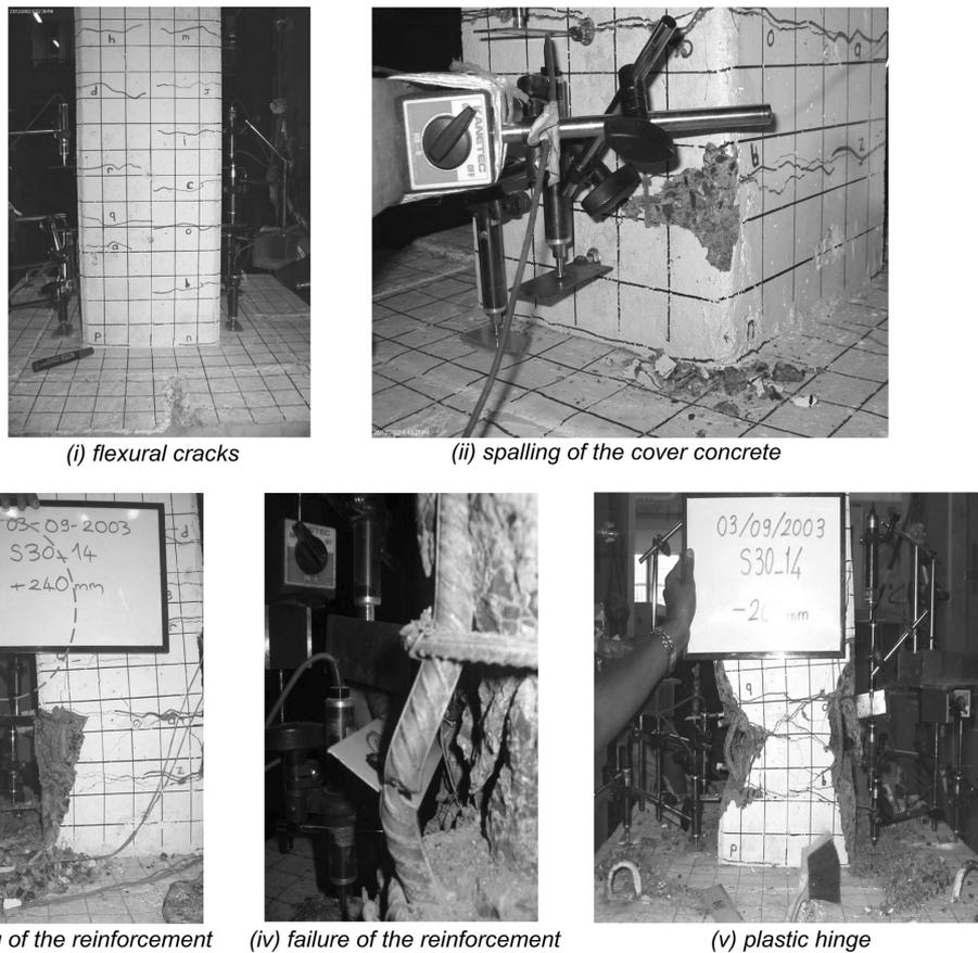
Fig. 5 Failed specimen S30-14
