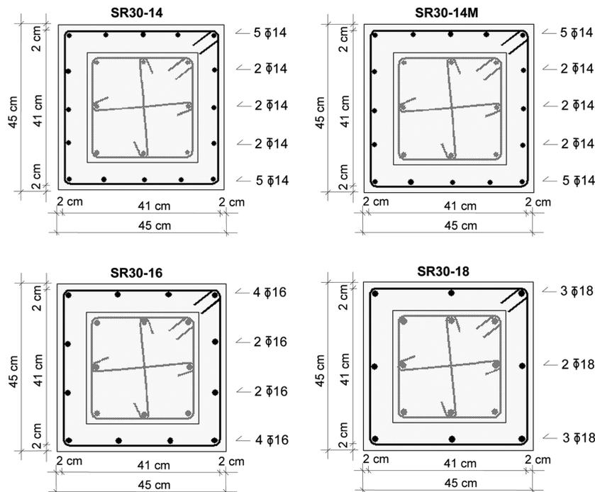
Fig. 7 Geometry and reinforcement details of jacketed columns
