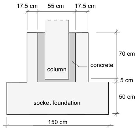
Fig. 1 Geometry of the socket foundation
