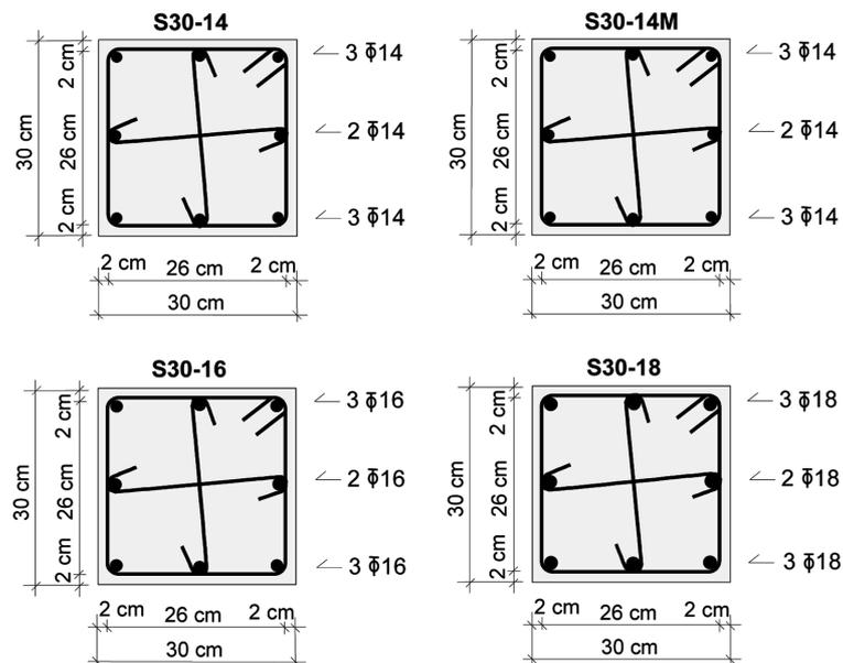
Fig. 2 Geometry and reinforcement details of original columns
