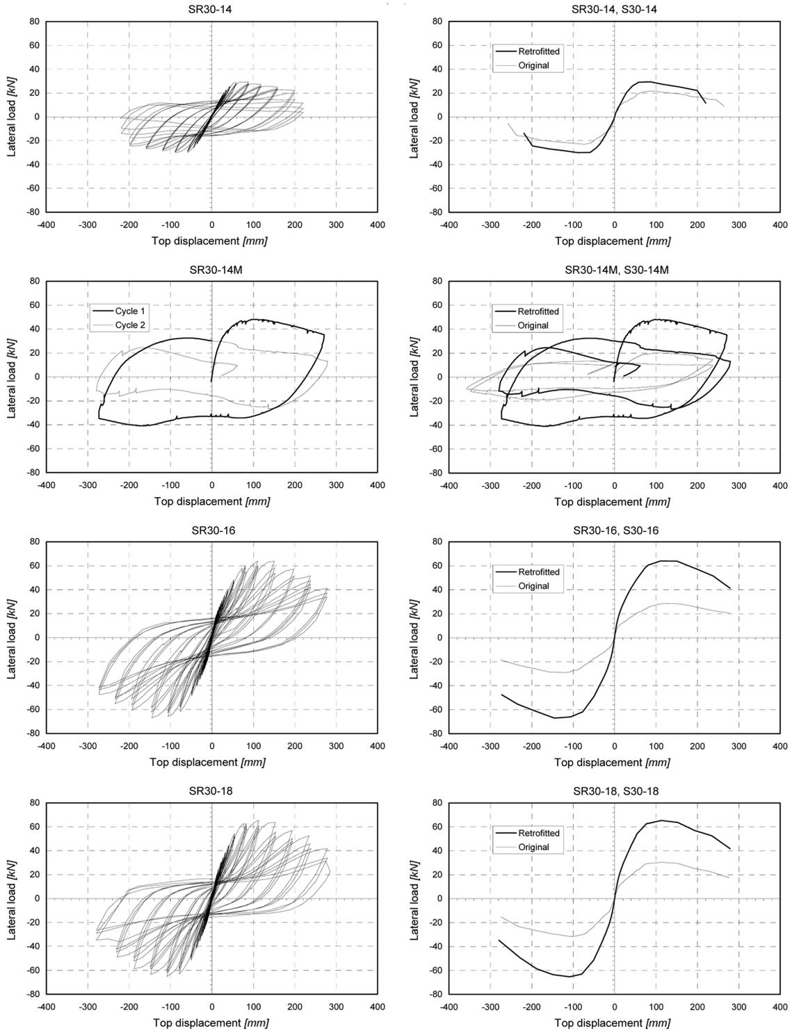
Fig. 12 Lateral load-top displacement curves of jacketed and original columns
