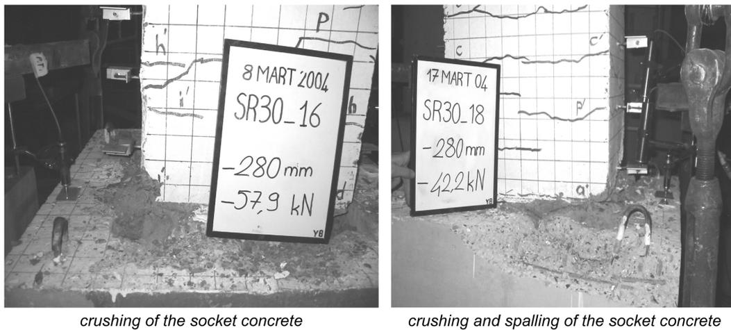
Fig. 10 Significant on specimens SR30-16 and SR30-18
