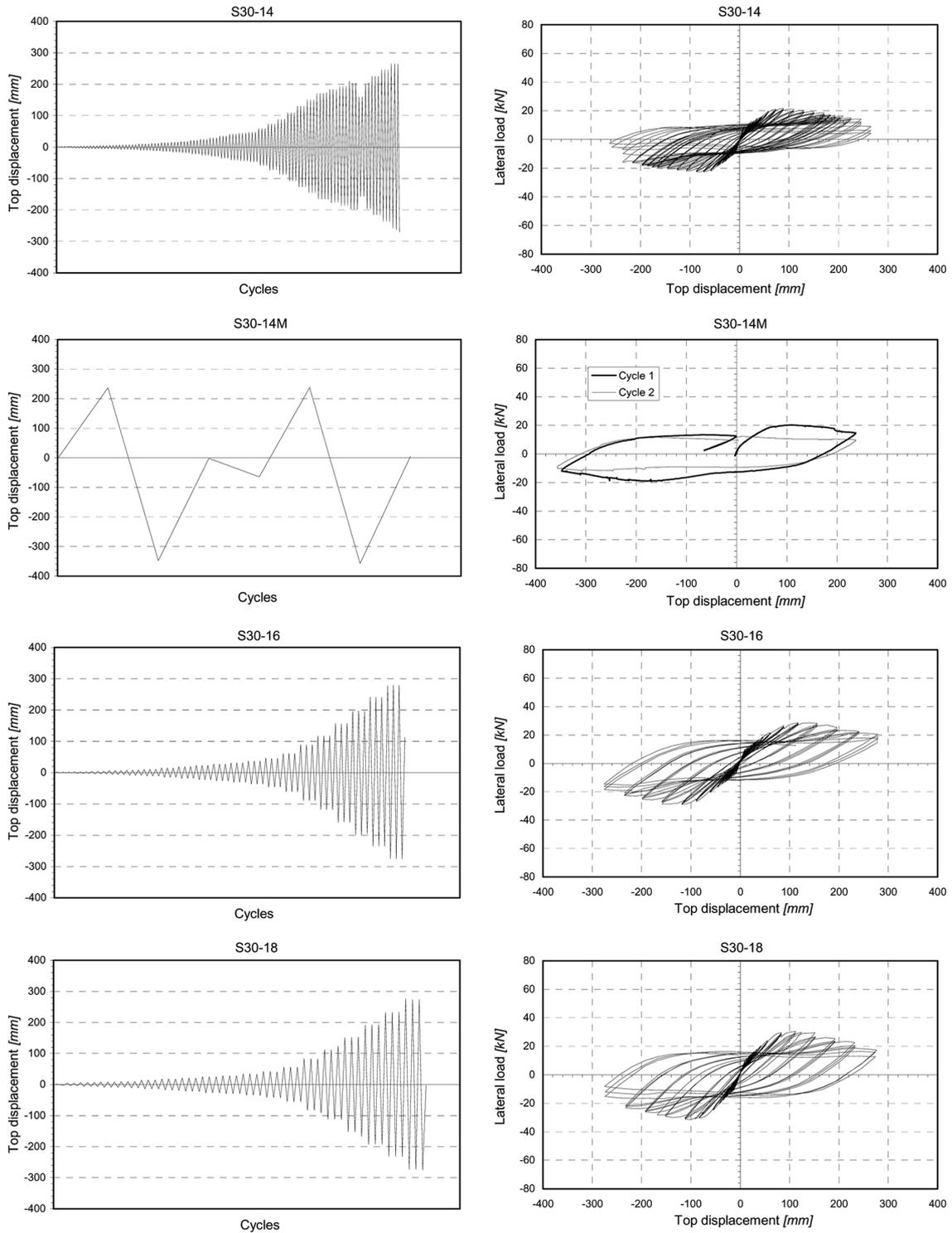
Fig. 6 The applied displacement cycles and response of the original columns
