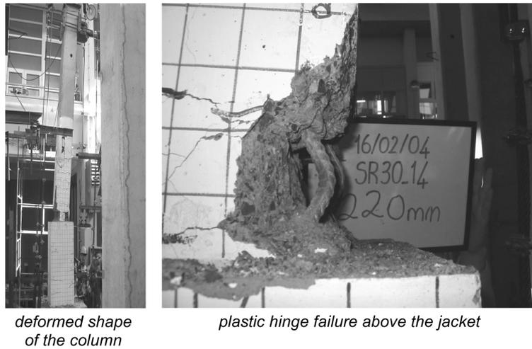
Fig. 9 Failed specimen SR30-14
