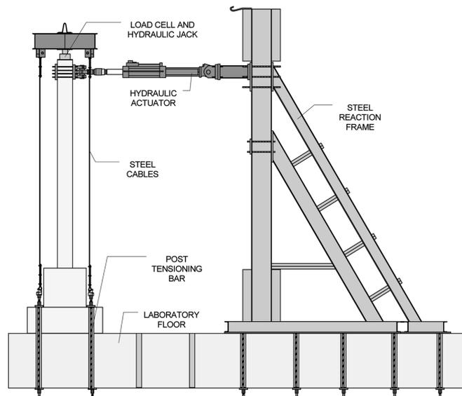
Fig. 3 Loading setup
