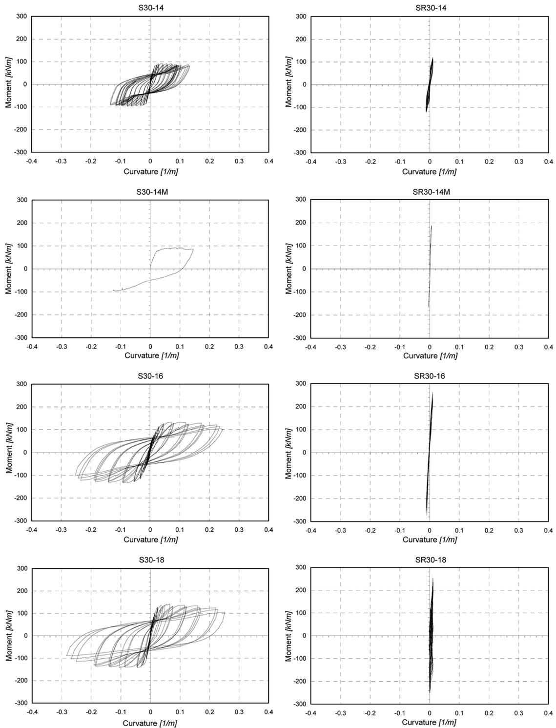
Fig. 11 Experimentally determined moment-curvature relations for the bottom edge of the columns
