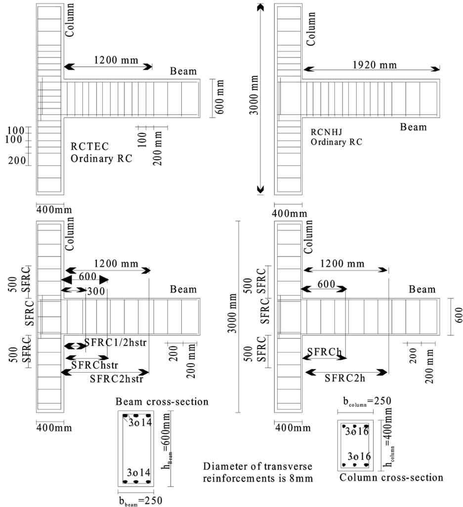
Fig. 1 Geometry and details of the test specimens
