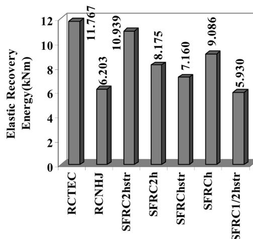
Fig. 11 Stored energy capacities of the specimens
