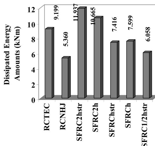
Fig. 10 Amounts of dissipated energy for each specimen
