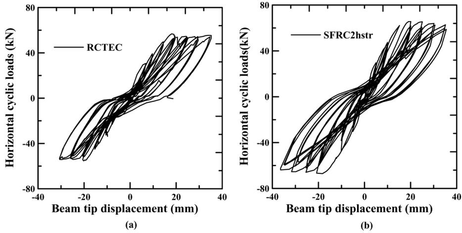
Fig. 4 Horizontal loads versus tip displacement hysteresis loops of the beam for RCTEC and SFRC2hstr
