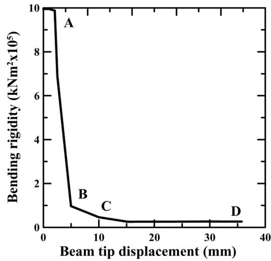
Fig. 13 Typical variation of the bending rigidity and displacement level of the beam plastic hinge zone in the beam-column joints subjected to the reversible cyclic loads
