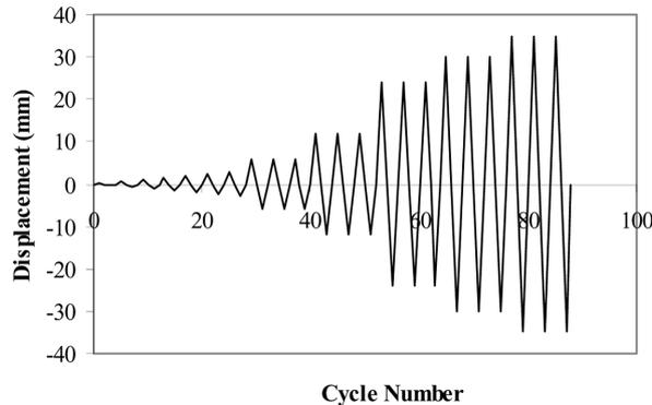
Fig. 3 Displacement controlled cyclic loading
