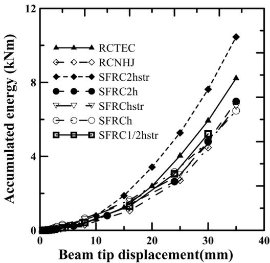
Fig. 8 Variation of the accumulated energy as a function of beam tip displacement for all specimens
