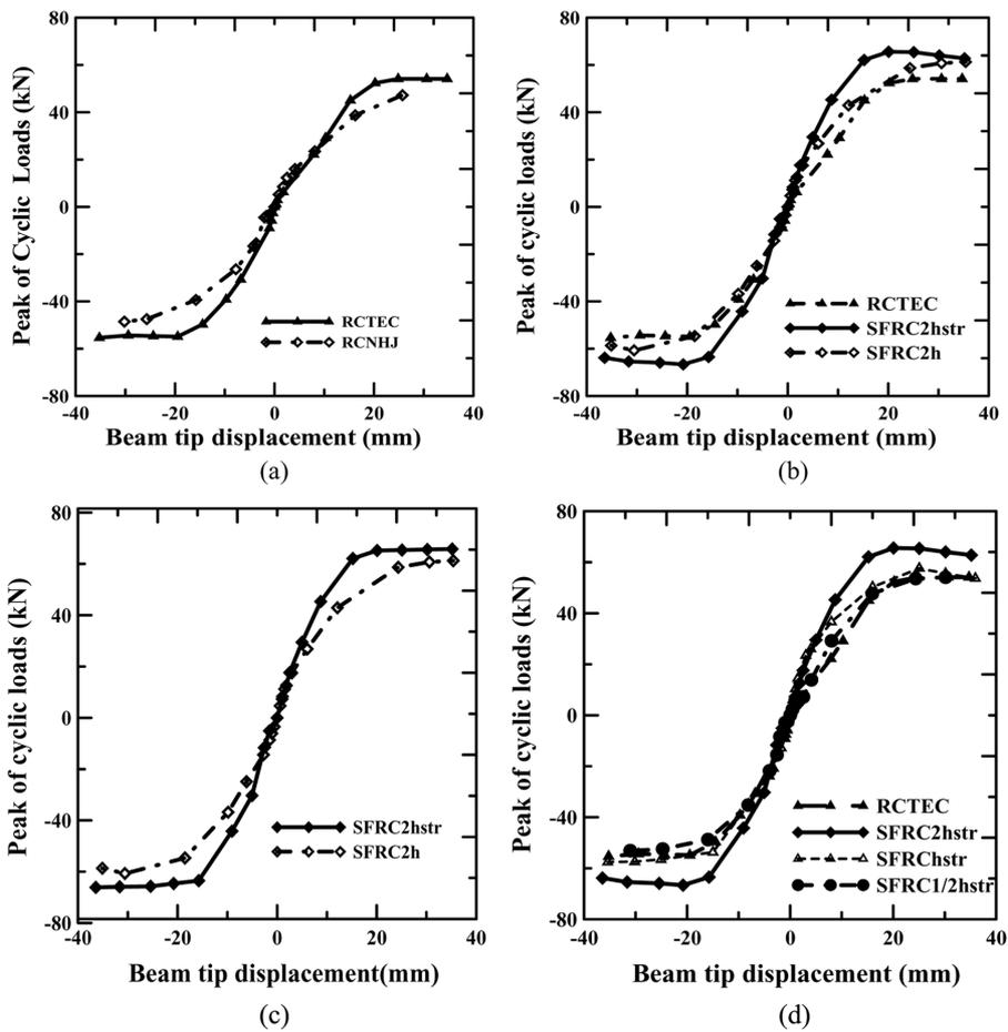
Fig. 5(a)-(d) Horizontal reversible cyclic loads versus tip displacements envelopes of the beam for selected specimens
