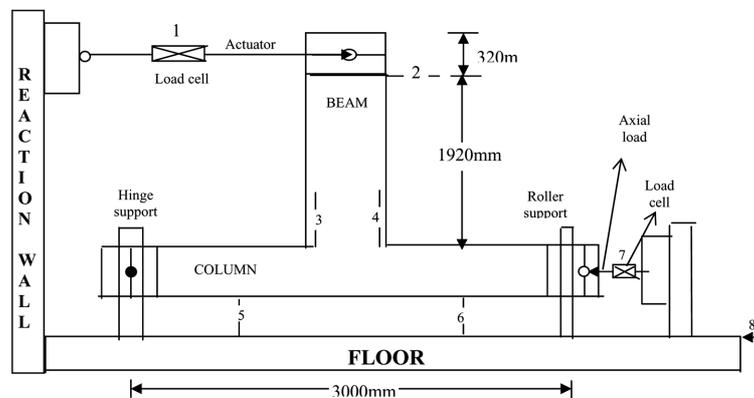
Fig. 2 General arrangement of the experimental set up and the beam tip displacement transducers
