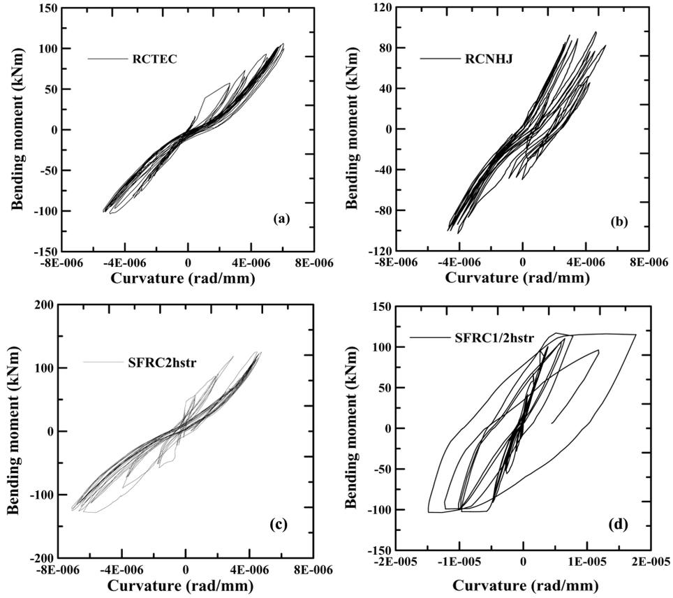
Fig. 12(a)-(d) Moment - curvature hysteresis loops of the selected specimens
