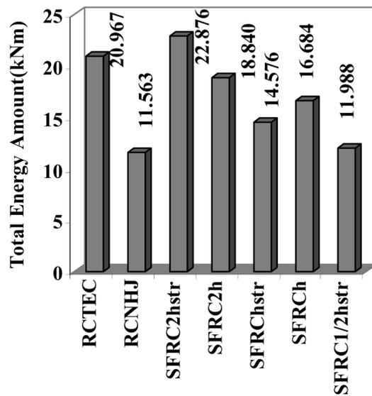
Fig. 9 Total energy capacities of the specimens
