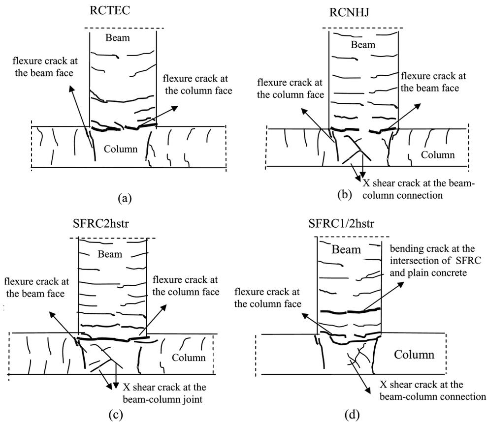
Fig. 6 Crack propagation of some specimens in the joint and the confinement regions of the beam and column
