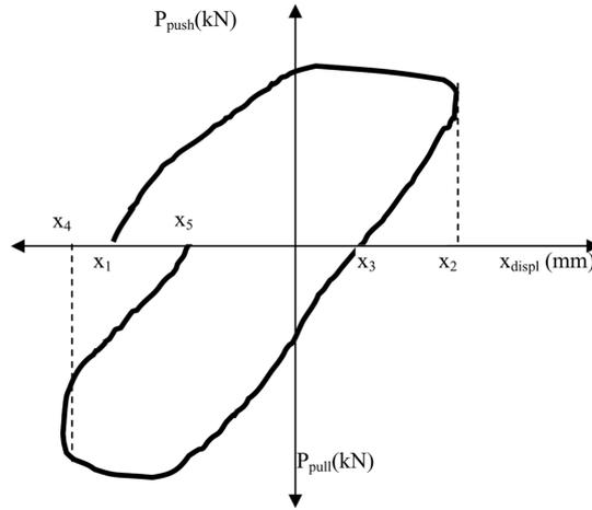
Fig. 7 Algorithm for the evaluation of energy and equivalent damping ratio for a beam tip load-displacement hysteresis loop model
