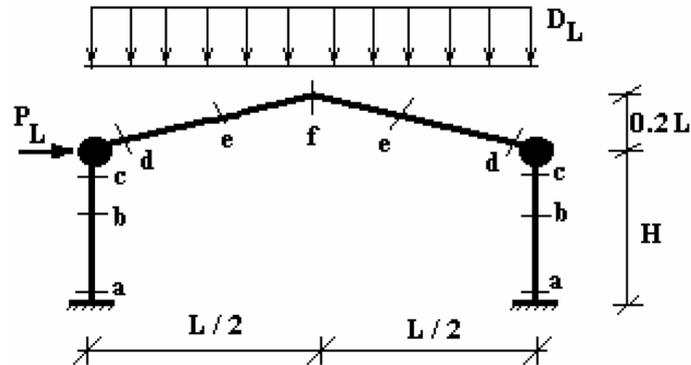
Fig. 6 Critical section of the sample frame and geometrical properties
