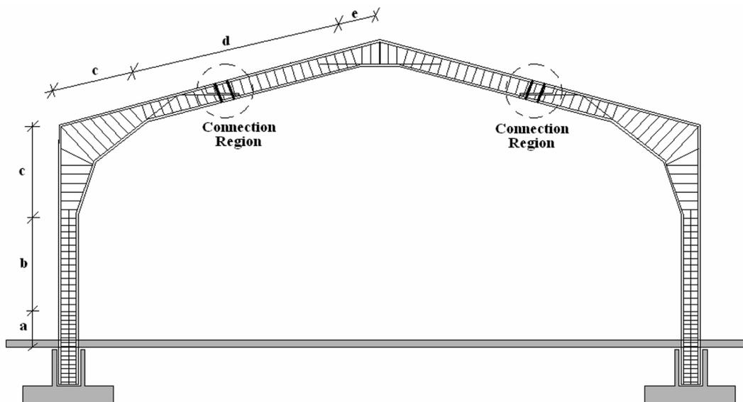
Fig. 7 Reinforcement details of the sample frame and its connection regions
