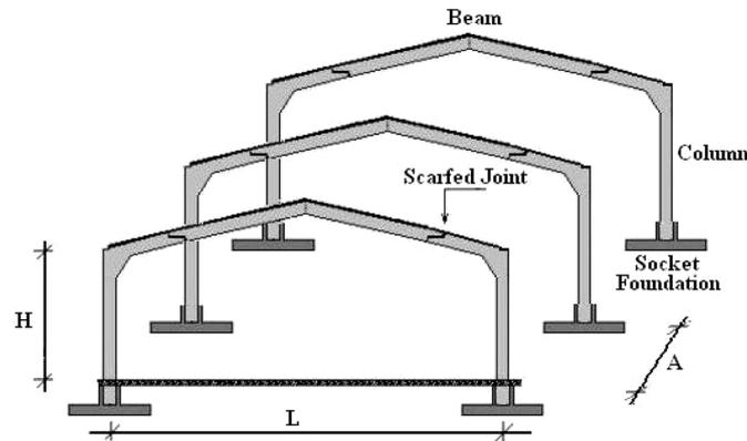
Fig. 5 Isometric (three dimensional) aspect of sample structure type
