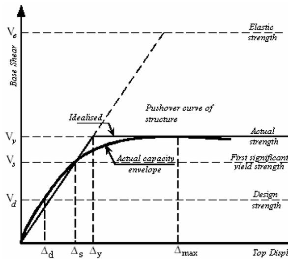
Fig. 1 Load displacement curve of a frame (Elneshai 2001)
