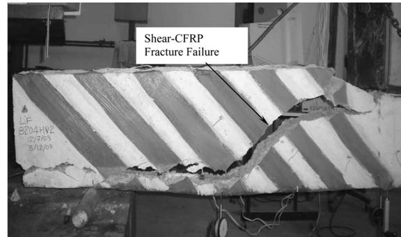
Fig. 3(f) Shear with CFRP fracture failure pattern for precracked/repaired beam BT2-2 (45/135 degree)
