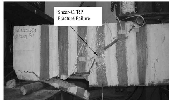
Fig. 3(b) Shear with CFRP fracture failure pattern for precracked/repared specimen BT1-1
