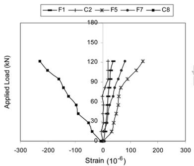
Fig. 5(e) Load versus surface strain in CFRP strip and concrete surface for precracked/repaired specimen BT2-2
