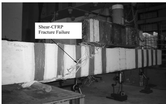
Fig. 3(c) Shear with CFRP fracture failure pattern for precracked/repared specimen BS1-2
