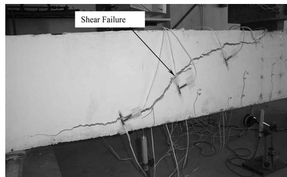
Fig. 3(d) Shear failure pattern for control specimen BT2a
