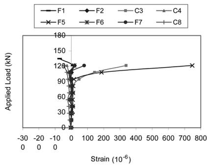
Fig. 5(a) Load versus surface strain in CFRP strip and concrete surface for precracked/repaired specimen BT1-1
