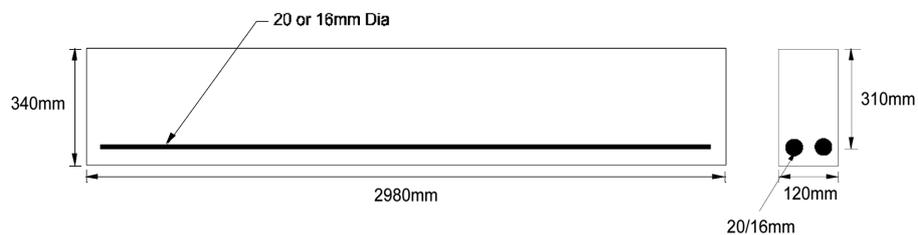
Fig. 1 Reinforcement details of series BT1/BT2/BS1/BS2
