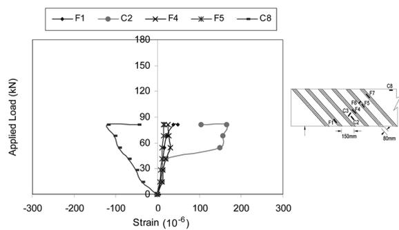
Fig. 5(f) Load versus surface strain in CFRP strip and concrete surface for precracked/repaired specimen BS2-2
