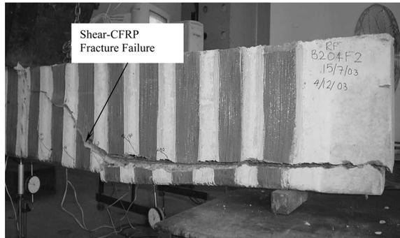
Fig. 3(e) Shear with CFRP fracture failure pattern for precracked/repaired specimen BT2-1
