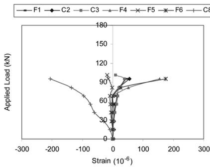
Fig. 5(c) Load versus surface strain in CFRP strip and concrete surface for precracked/repaired specimen BS1-2
