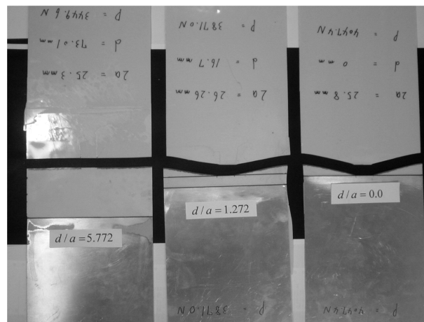
Fig. 2 Fracture patterns ( d/a = 0.0 , 1.272, 5.772)
