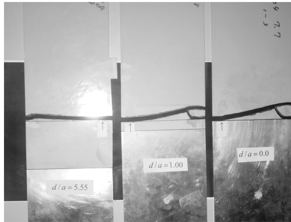
Fig. 10 Fracture patterns ( d/a = 0.0, 1.0, 5.55 )
