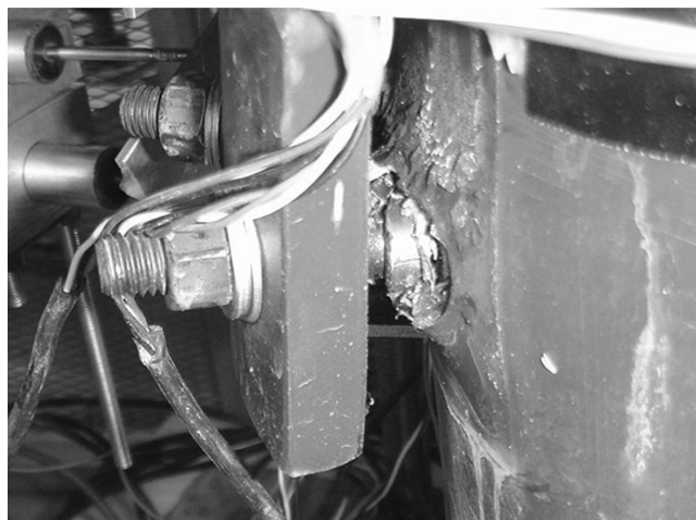
Fig. 8 Brittle failure of Specimen 1
