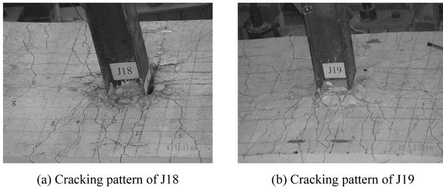
Fig. 8 Cracking pattern of concrete slab
