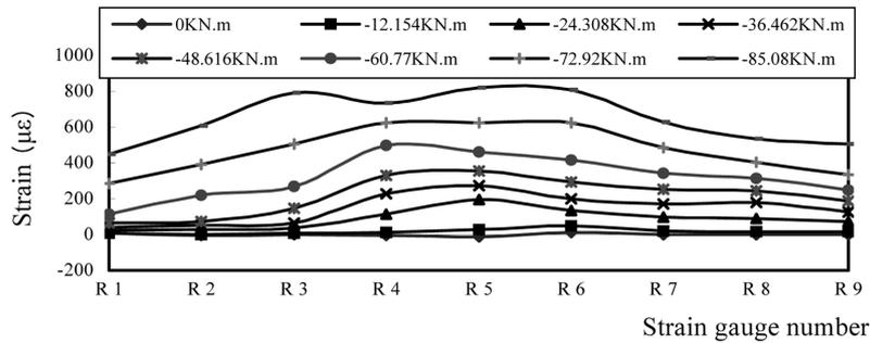
Fig. 14 Strain distribution on slab reinforcements in J19 under negative moment
