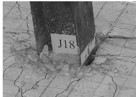
Fig. 12 Crush of concrete around column
