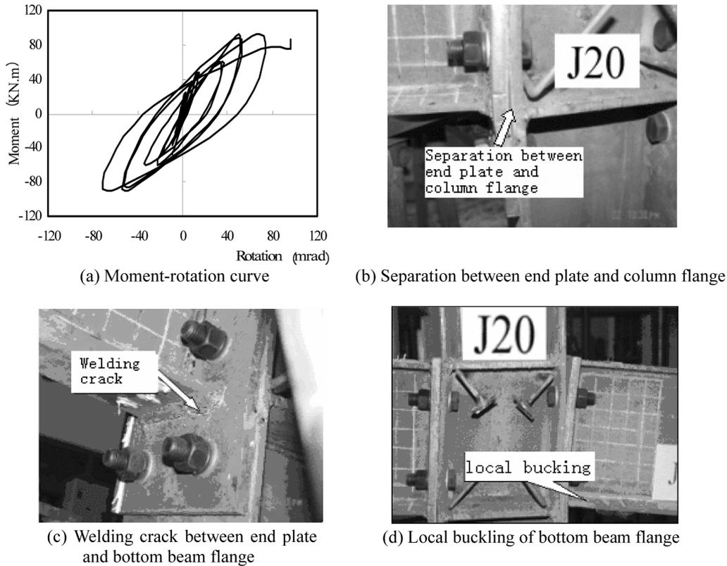
Fig. 6 Test results of specimen J20
