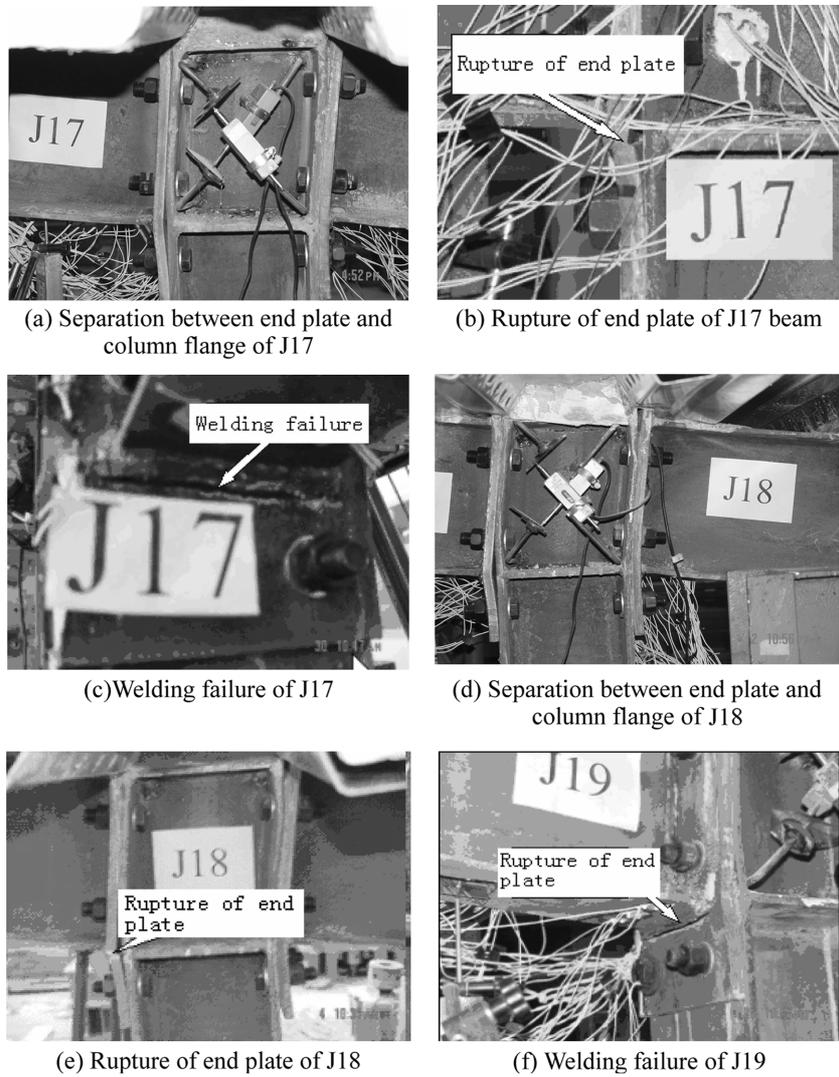
Fig. 10 Test results of end plate in specimen J17, J18 and J19
