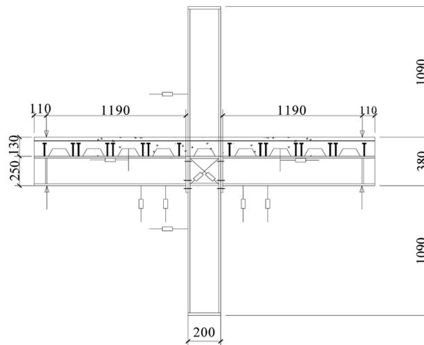
Fig. 5 Arrangement of transducers
