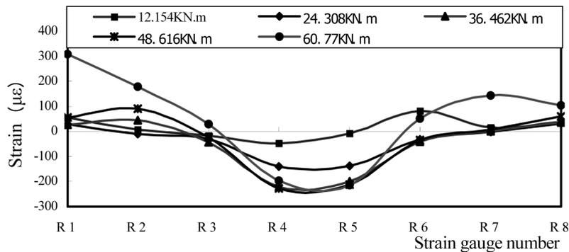
Fig. 13 Strain distribution on slab reinforcements in J17 under positive moment
