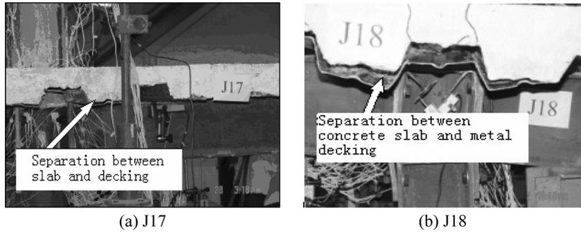
Fig. 9 Separation between concrete and metal decking
