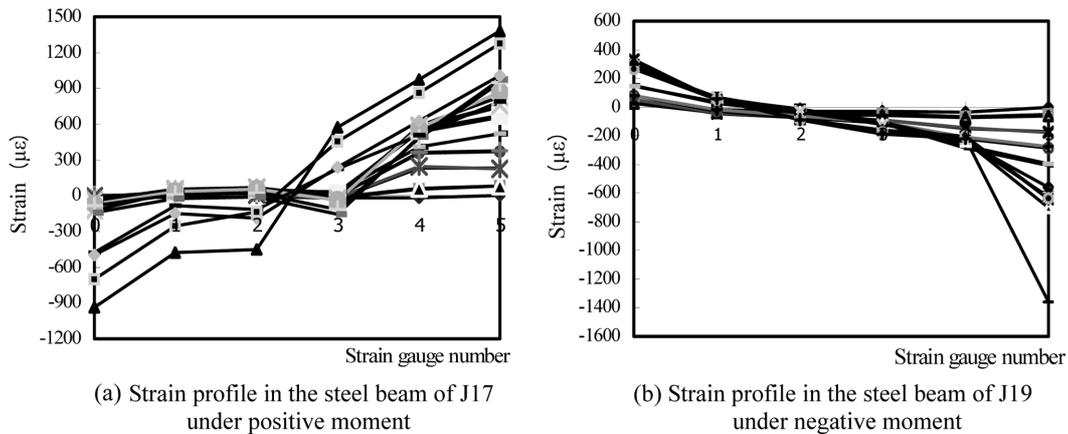
(a) Strain profile in the steel beam of J17 under positive moment
