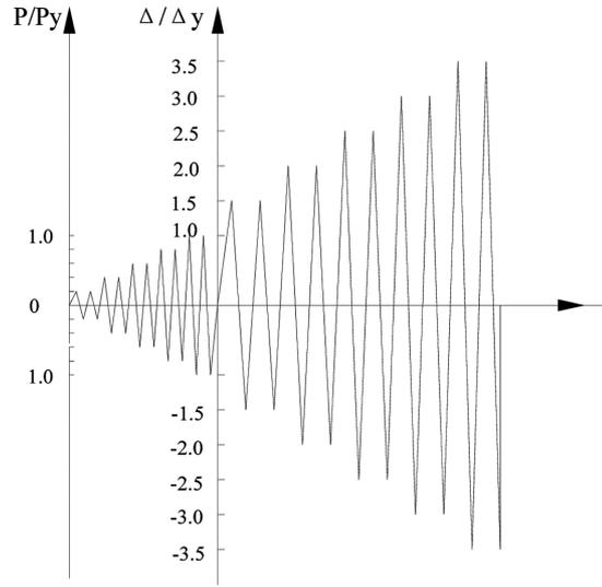
Fig. 3 Typical loading procedure for cyclic test
