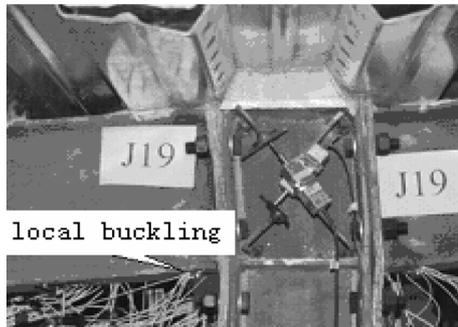
Fig. 11 Local buckling of beam bottom flange
