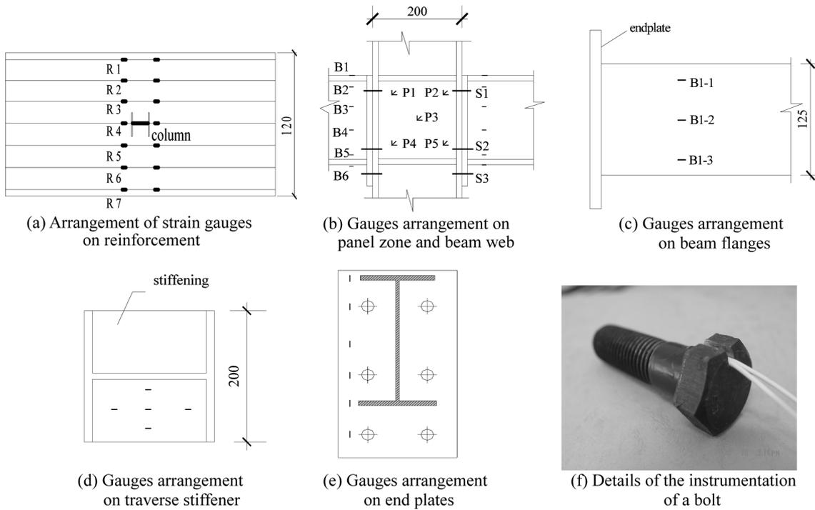
Fig. 4 Gauges arrangement on crucial locations
