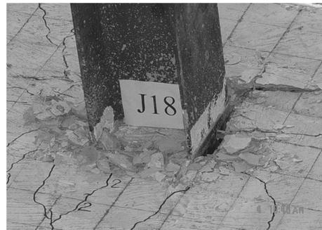
Fig. 12 Crush of concrete around column
